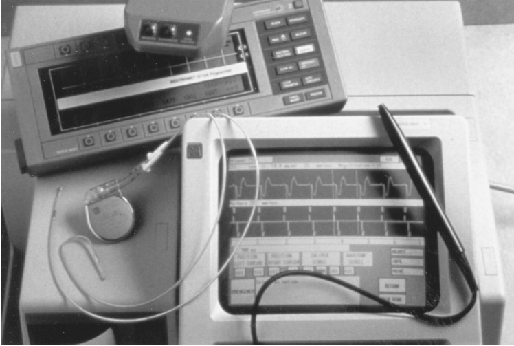
FIGURE 54.1 The pacing systems comprise a programmer, pulse generator, and lead. There are two programmers pictured above; one is portable, and the other is an office-based unit.
