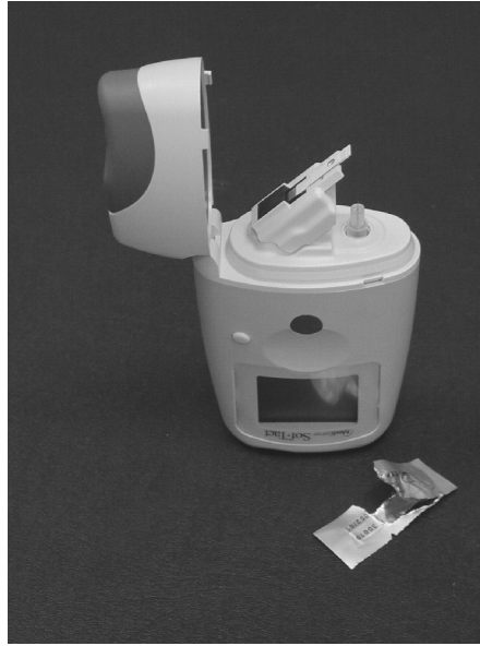
FIGURE 66.3 Sof-Tact meter with cover opened to load test strip and lancet. Test strip is inserted into an electrical connector. The hole in the opposite end of the test strip allows the lancet to pass through. The white cylindrical lancet is loaded into the lancet tip holder in the housing. To perform a test, the cover is closed, the gray area of the cover placed against the skin and blue button depressed.
