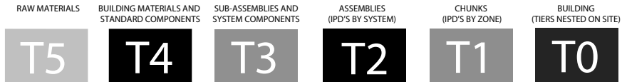
Figure 9.2 New tiers expressing the system levels of the system structure model [Author's drawing]
