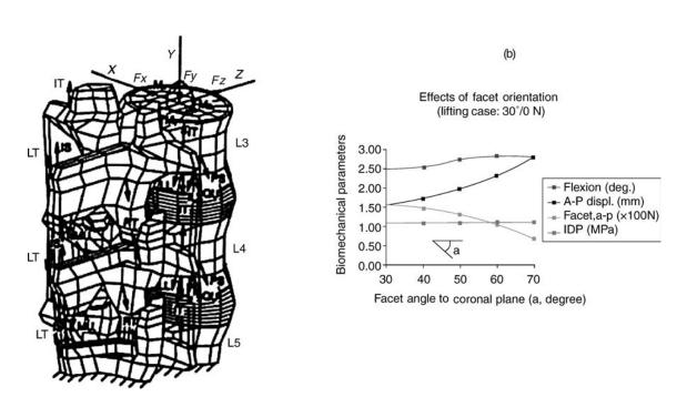
**Figure 11.** The finite element of a lumbar segment used to predict the effect of facet orientations on the motion and loads in various spinal components in a motion segment. (Taken from Ref. 77.)
