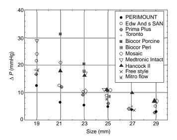
**Figure 9.** In Vitro pressure drop data of various prosthetic aortic valves. (Reprinted with permission from *The Journal of Heart Valve Disease.*)
