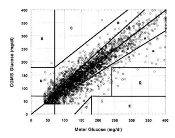
**Figure 7.** An approach to sensor validation. Comparison of 2477 glucose values determined by a CGMS sensor system and a standard meter (63). Data pairs were collected during home use from 135 patients. The plot, known as the Clarke Error Grid, has zones with differing clinical implications. This type of plot is widely used to describe glucose sensor performance, but has limited ability to discriminate ineffective sensors (64). (Copyright © 1999, Elsevier.)
