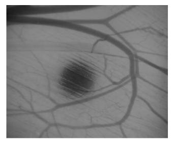
Figure 12. An implanted glucose sensor and nearby microvasculature (79). Optical image taken in a hamster window chamber. Sensor diameter is  $125 \,\mu$ m.
