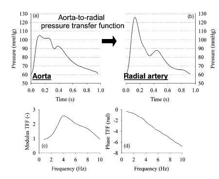
**Figure 12.** Demonstration of the aorta-to-radial pressure pulse amplification: (a and b) are carotid (as substitute for aorta pressure) and radial artery pressure measured in the same subject with applanation tonometry (1 mmHg = 133.3 Pa). (c and d) Display the modulus and phase angle of the radial-to-aorta transfer function as published by Ref. (99).
