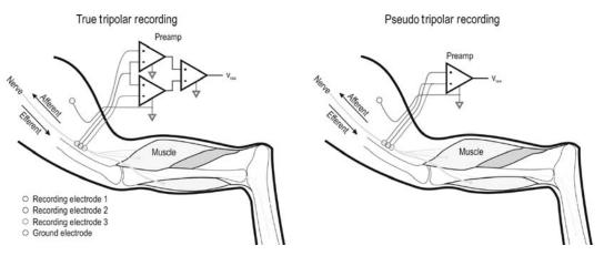
**Figure 10.** Tripolar recording configurations. (Left panel) Shows the true tripolar recording configuration consisting of a double differential amplification circuit. (Right panel) Shows a pseudo-tripolar recording technique, which approximates the true tripolar recording configuration by shorting the outer two electrodes 1 and 3.
