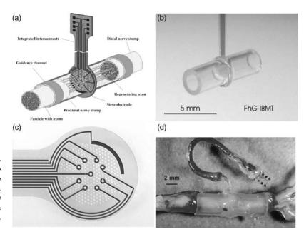
**Figure 18.** (a) Sketch of a Sieve electrode. The proximal and distal nerve stumps are fed into a guide tube. Neural axons must grow through holes in the Sieve electrode to reconnect with the neural axons on the other side. (b,c) Examples of Sieve electrodes. (d) shows the Sieve electrode *in situ*. (Reproduced with permission from T. Stieglitz, Fraunhofer Inst., Germany.)
