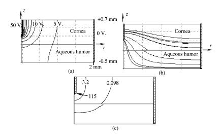
**Figure 26.** Needle electrode in cornea, FEM model results. Cornea conductivity  $1.125 \,\mathrm{S \cdot m^{-1}}$ , aqueous humor  $1.5 \,\mathrm{S \cdot m^{-1}}$ . (a) Potential field V(r,z) for 50 V (rms) electrode potential. (b) Electric field stream-lines. (c) Volume power density with contours at 115, 3.2, and  $0.098 \,\mathrm{kW \cdot cm^{-3}}$ .
