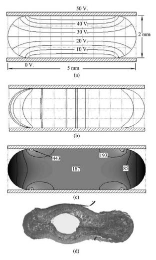
**Figure 27.** Bipolar forceps applied to a vessel, FEM model results. (a) Potential field, V(x,y) for 50 V(rms) electrode potential. (b) Electric field streamlines. (c) Volume power density,  $q_{\text{gen}}$ , with contours at 85, 193, and 443 (W·cm<sup>-3</sup>). (d) Typical result: canine femoral artery temperature 89 °C for 2 s (thermocouple in center of artery; original magnification  $40\times$ , Mallory's trichrome stain).
