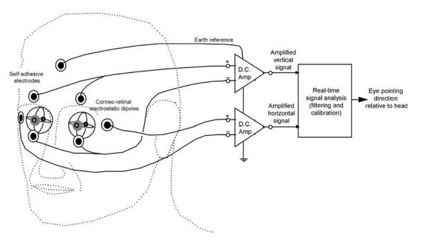
**Figure 4.** Schematic illustrating the EOG method of measuring eye movement. (Adapted from a diagram in Ref. 8.)
