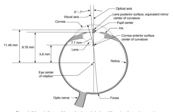
**Figure 1.** Schematic diagram of the eye showing typical values of dimensions that are important in eye movement measurement. The dimension values, which do vary between individuals, are derived from Refs. 1 and 2.
