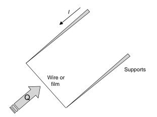
Figure 8. Illustration of a hot wire or film element.
