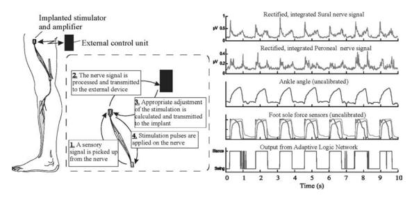
**Figure 26.** Footdrop correction system, using natural sensory information from the Sural or Peroneal nerve. The nerve signals were processed to determine heel contact with the floor and to decide the timing of the ankle dorsi-flexion stimulation. The stimulation may be applied through a peroneal nerve cuff electrode innervating the Tibials Anterior muscle or by surface electrodes. (Reproduced with permission from Dr. T. Sinkjær, Dr. M. Haugland, and Dr. M. Hansen.)
