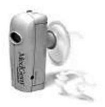
**Figure 15.** A simple oxygen-uptake monitor. The subject wears the mask and a small ultrasonic flow meter measures the respiratory volume and a fluorescence oxygen monitor measures the oxygen concentration. This device is only used for measuring basal metabolism.
