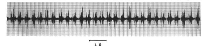
**Figure 5.** Illustration of the raw reflected ultrasound signal from the beating fetal heart *in utero*. Note that two ultrasonic bursts occur per cardiac cycle.
