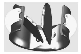
**Figure 5.** A cut-away view of the On-X valve showing leaflets in the closed (left) and open (right) positions. The valve orifice or annulus ring has pivot depressions in the inside diameter wall and is encased in a sewing cuff. The orifice wall has a bulge and two external metal wires for stiffening.
