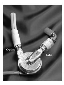
**Figure 10.** Thoratec HeartMate III Centrifugal Flow Ventricular Assist Device. The HeartMate III is a centrifugal pump that features a magnetically levitated impeller. (Reprinted with permission from Thoratec Corporation.)
