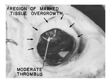
**Figure 8.** Photograph of an explanted mechanical heart valve prosthesis with thrombus deposition on the leaflet surface and tissue ingrowth (Courtesy of Prof. Ajit Yoganathan of Georgia Institute of Technology, Atlanta, GA.)
