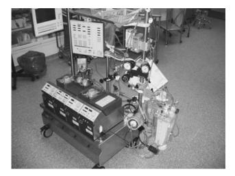
**Figure 2.** Typical cardiopulmonary bypass circuit demonstrating the various components. This circuit contains four accessory pumps for suction/venting and the administration of cardioplegia. (Reprinted with permission from Ref. 13.)
