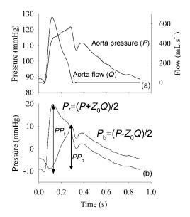
**Figure 9.** Application of linear wave separation analysis to the pressure (1 mmHg = 133.3 Pa) and flow data of Fig. 1. The ratio of  $PP_b$  and  $PP_f$  can be used as a measure of wave reflection magnitude.
