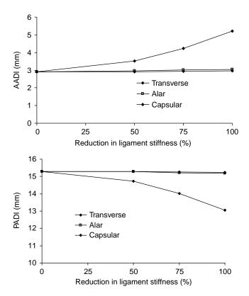
**Figure 10.** (a) Anterior atlantodental interval (AADI) (b) and posterior atlantodental interval (PADI) calculated for the intact model and models with stiffness reductions of the transverse, alar, and capsular ligaments at the fully flexed posture (1.5 N·m moment load). Each ligament's stiffness was altered while holding the other two at the baseline value (completely intact). (Taken from Ref. 66.)
