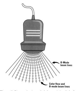
**Figure 15.** Diagram showing method of transmission of color flow Doppler ultrasound signals. Packets or ensembles of pulses represented by the open circles in the figure are sent out along some of the scan lines of the image. The reflected waves are analyzed in an autocorrelation circuit to allow display of the color flow image. (Reprinted from Zagzebski JA. Essentials of Ultrasound Physics. St. Louis: Mosby-Year Book Inc. copyright © 1996, with permission from Elsevier.)
