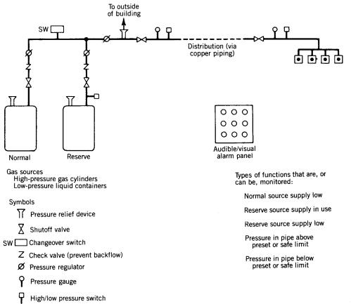
**Figure 1.** Components of a medical gas (pressurized) central piping system (simplified). Standards have been developed for component and total-system performance and safety.
