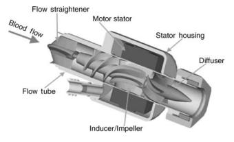
**Figure 13.** MicroMed Debakey Axial Flow Ventricular Assist Device. The MicroMed is connected to an external controller and power unit. The pump speed is varied manually to meet the needs of the patient. (Reprinted with permission from Micromed Technology, Inc.)
