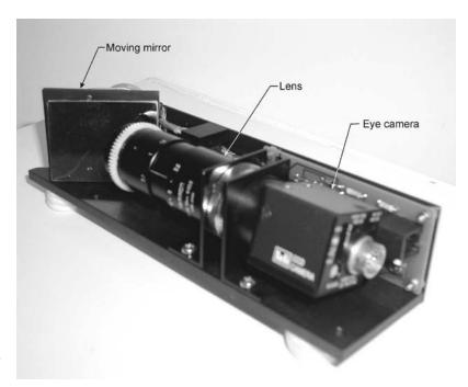
**Figure 20.** Example of a remote eye tracker optics module that uses a moving mirror to keep a telephoto eye image within the camera field of view. The optics module is shown with its cover removed. (Courtesy of Applied Science Laboratories, Bedford, MA.)
