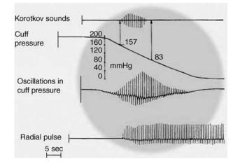
**Figure 3.** Principle of the oscillometric method. The pulsations induced by the artery differ when the artery is compressed. Initially, no pulsation occurs, and then the pulsation starts. As the pressure decreases in the cuff, the oscillation becomes more significant, until the maximum amplitude of the oscillations defines the average blood pressure. Then, the oscillations decrease with the cuff pressure until they disappear.
