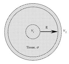
**Figure 22.** Geometry for coaxial cylinder electrode example. The outer cylinder typically comprises the return electrode,  $V_2 = 0$ .
