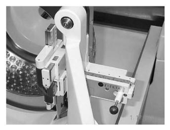
Figure 10. Close-up view of trunnions and helmet of Leksell Gamma Unit model C with Automatic Positioning System in place.
