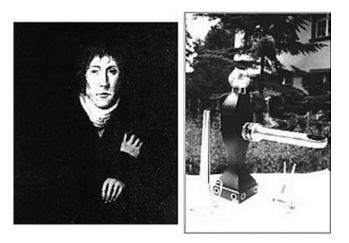
Figure 1. Phillip Bozzini's Lichtleiter endoscope.
