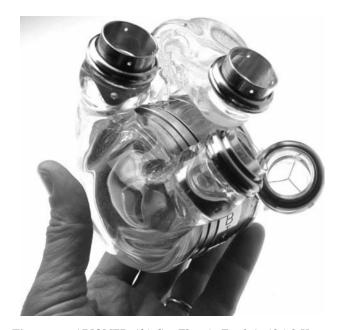
**Figure 18.** ABIOMED AbioCor Electric Total Artificial Heart. The AbioCor TAH uses an electro hydraulic energy converter to alternately compress each blood sac. The AbioCor is currently undergoing clinical trials in the United States. Two patients were discharged from the hospital, with one patient surviving for > 1year. (Reprinted with permission from ABIOMED, Inc.)
