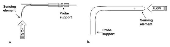
**Figure 1.** Examples of invasive velocity measurement sensors with displaced sensing elements relative to their probe supports. (a) a boundary layer style hot-wire probe for thermal anemometry. Picture from TSI Inc. catalog, probe catalog 1261A. (b) Pitot static probe for velocity measurement.
