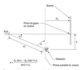
**Figure 11.** Relationship, in one plane, between point-of-gaze on a flat scene and relative eye, detector, and scene positions. (From Ref. 26.)
