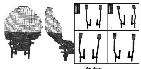
**Figure 15.** The finite elment model showing the posterior fixation system and the stress plots in the rods. (Taken from Ref. 4c.)
