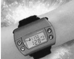
**Figure 13.** Glucowatch device (1) and principle of iontophoresis (2). This device provides noninvasive monitoring of glucose and uses reverse iontophoresis to extract glucose from the skin to monitor glucose. A low electric current is applied, which draws interstitial fluid through the skin. The glucose in this fluid is collected in a gel. A chemical process occurs, which generates an electrical signal that is converted into a glucose measurement.
