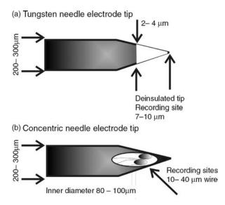
**Figure 19.** Microneurography electrodes. (a) A drawing of the geometry of a typical, commercially available tungsten needle electrode. A separate ground or indifferent electrode must be place in the close surroundings (Drawings appear courtesy of Dr. K. Yoshida.) (b) A drawing of a concentric needle electrode. One or two fine wires are threaded through a hypodermic needle and attached
