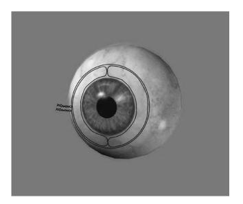
**Figure 3.** Schematic showing the configuration of the second coil in a dual induction coil system. The second coil forms a loop whose enclosed area has a component parallel to the optical axis of the eye (perpendicular to the plane of the pupil), and is used to measure torsional movement. Although the diagram shows only one winding for each coil, the actual device uses multiple windings.
