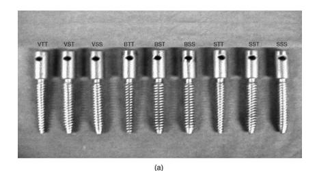
Figure 14. (a) Types of screws used in the foam model to determine the pull-out strength. The nomenclature used is as follows: Square = S, Buttress = B, V-shape = V. Screw diameters were SS = straight major diameter on straight core, ST = straight major diameter on tapered core, TT = tapered major diameter on tapered core. (b) Regression analysis. The maximum and minimum values from pull-out test for each foam grade were used regardless of tooth or core profiles. (Taken from Ref. 112.)
