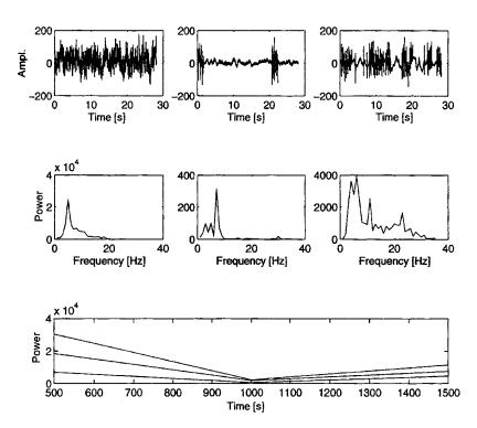
**Figure 10.** STFT. (a) Epoch of an EEG signal recorded from an isoflurane/DEX-treated dog. The time-varying character of this signal can be presented in the power spectrum using the STFT as shown in (b).STFT was performed with a 256 point FFT and a window length (Hamming window) of 128 points with an overlap of 50%. Data were sampled at f = 250 samples.
