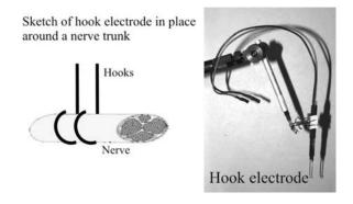
**Figure 24.** A hook electrode consists of two simple wires/hooks that are held in close contact with the nerve surface. The picture shows an example of a custom made hook electrode. (Courtesy of Dr. K. Yoshida, Aalborg University, Denmark.)
