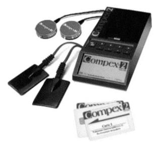
**Figure 4.** The Compex Motion FES system, manufactured by the Swiss based company Compex SA, is a general purpose programmable transcutaneous electrical stimulation device. Seen are the stimulator unit, three memory chip-cards that are inserted into the stimulator and used to store all pertinent information for a specific protocol, two EMG sensors, and two surface electrodes. (Reprinted from Ref. 83 with permission from the Institute of Physics and Engineering in Medicine.)
