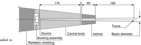
Figure 11. Geometry of sources installed in Leksell Gamma Units.
