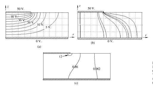
**Figure 25.** Circular disk electrode FEM model results. Muscle conductivity  $90.3 \,\mathrm{S} \cdot \mathrm{m}^{-1}$ . (a) Potential field, V(r,z). (b) Electric field streamlines. (c) Volume power density with contours at 0.062, 0.86, and  $12 \,\mathrm{W} \cdot \mathrm{cm}^{-3}$ .
