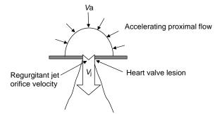
**Figure 9.** Illustration of the proximal isovelocity surface area (PISA) concept.
