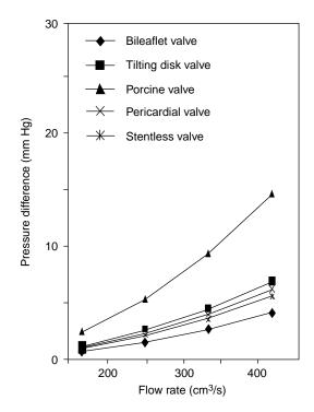
**Figure 11.** Typical plots for the pressure drop as a function of flow rate for the various mechanical and bioprosthetic valve prostheses (Courtesy of Prof. Ajit Yoganathan of Georgia Institute of Technology, Atlanta, GA.)
