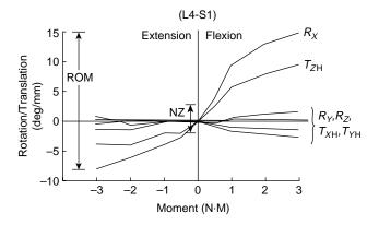
**Figure 6.** The load-displacement response of a FSU in flexion and extension. Two of the motion components are major and the other four are minor (or coupled). The range-of-motion and neutral zones, two of the terms used to describe the motion behavior of a segment, are also shown. (Adapted from Ref. 1.)
