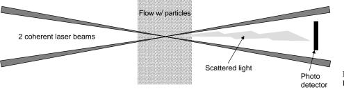
**Figure 12.** Illustration of the dualbeam or fringe mode LDV setup.
