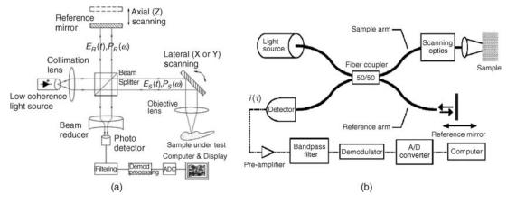
**Figure 10.** Optical coherence tomography (OCT). (a) Principle of OCT (From Wikipedia.org). (b) Possible implementation of fiber-based OCT (38).
