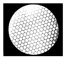
Figure 8. Cross-section of the imaging bundle.
