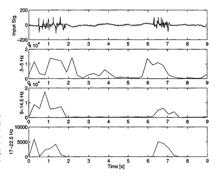
**Figure 11.** Energy profile in dominat frequency bands using the STFT. (a) EEG epoch recorded from isoflurane/DEX-treated dog. Summing together the energy in the frequency bands 0.5–5, 9–14.5, and 17–22.5 Hz, we obtain the energy profiles in the dominant frequency bands as shown in (b). Note that burst sequences and sequences of electrical silence in the EEG signal can be clearly distinguished with this method.
