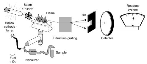
**Figure 4.** Components of a flame atomic absorption spectrometer.
