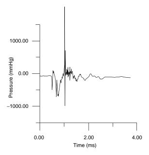
**Figure 16.** Typical negative pressure transients recorded at the instant of mechanical heart valve closure (in the mitral position) with the pressure transducer placed very close to the leaflet on the inflow side (atrial side) from *in vitro* experiments.
