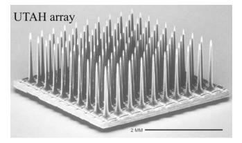
**Figure 21.** The 100-channel UTAH array. The electrode was originally developed at University of Utah, by Dr. R. A. Normann and colleagues. The electrode is commercially available through Cyberkinetics Inc. (Courtesy of Dr. R. A. Normann, University of Utah.)
