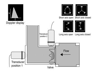
**Figure 11.** Ultrasound measurements in a pulse duplicator. In transducer position 1, the transducer is aligned with the flow and emits a sound wave that reflects off particles in the fluid; the return signal is measured by the transducer and the Doppler equation is used to calculate velocity. Transducer position 2 is used to obtain short-axis (cross-sectional) and long axis images of the valve as it opens and closes.
