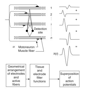
Figure 3. Schematic representation of the generation of the motor unit action potential.
