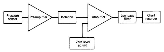
Figure 9. Block diagram of the signal processing electronics for intrauterine pressure measurement.
