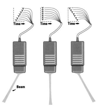
**Figure 9.** Diagram of a phased array transducer. Beam direction is varied by changing the delay sequence among the transmitted pulses produced by each individual element. (From Zagzebski JA. Essentials of Ultrasound Physics. St. Louis: Mosby-Year Book Inc.; copyright © 1996, with permission from Elsevier.)
