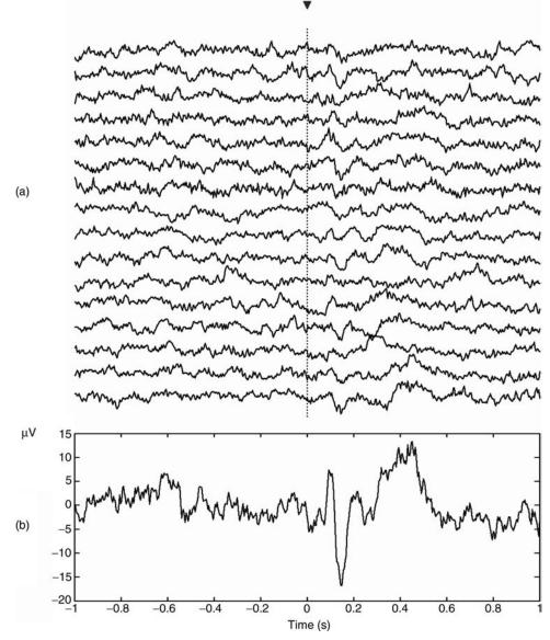
**Figure 4.** (a) Sixteen single-trial responses of a typical subject and (b) the average response. The triangle marks the time of stimulation. Note that the evoked responses are clearly seen after averaging, but are hardly identified in the single trials.
