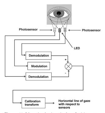
**Figure 14.** Schematic showing simple reflectivity pattern (limbus) tracker for horizontal measurement. (Adapted from a diagram in Ref. 8.)
