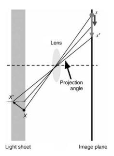
**Figure 21.** Illustration of the perspective projection; the red arrow is the vector obtained from perspective projection, the blue is the correct projection of displacement vector on the *XY* plane (68).
