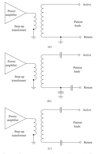
**Figure 9.** Generator output impedance matching circuits. The step up transformer is used to achieve higher open circuit output voltages. (a) grounded, (b) referred-to-ground, (c) isolated.
