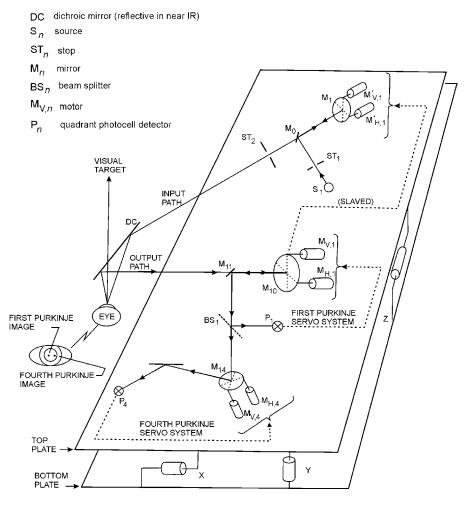
**Figure 15.** Schematic representation of Double Purkinje image eye tracker. (Redrawn from Ref. 73.)
