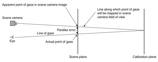
**Figure 12.** Parallax error when gaze direction is mapped (calibrated) to a scene camera image plane that is different from the plane being fixated.
