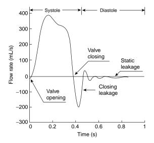
**Figure 12.** Flow rate across mechanical valve prosthesis in the aortic position obtained in a pulse duplicator *in vitro* measured with an electromagnetic flow meter.
