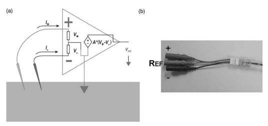
**Figure 6.** (a) Shows a schematic representation of the differential preamplifier and its electrode connections when used as a bioamplifier on tissues. (b) Shows a low noise differential preamplifier that could be used to record neural activity with a low impedance electrode.
