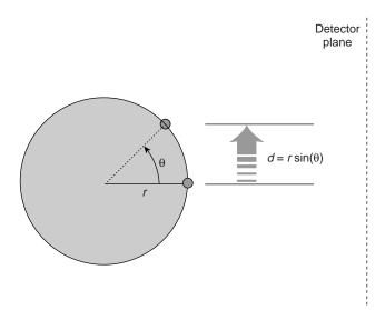
**Figure 7.** Schematic illustrating the principle behind single feature tracking. Observation of a single land mark on the sphere allows determination of its orientation, so long as the center of the sphere does not move.
