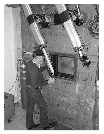
**Figure 7.** Loading cobalt-60 sources into Gamma Unit with remote manipulating arms.
