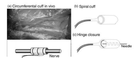
nerve trunk and to achieve a good signal/noise ratio. The cuff tube or wall is made of a flexible, biocompatible material, such as silicone, (1,64,65) or polyimide (66,67). The cuffs may be handmade or microfabricated. The microfabrication technique has the advantage that thinner walls can be obtained.
