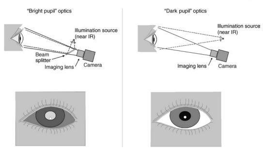
Figure 6. Illustration of bright and dark pupil optics. In the bright pupil example, retroreflected light from the retina will beam back into the camera lens, resulting in a bright, back lit, pupil image.
