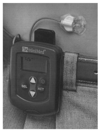
Figure 6. Components of the MiniMed CGMS system (62). This sensor, based on the peroxide-based sensing principle, is FDA approved for short-term monitoring. (Copyright © 1999, Elsevier.)
