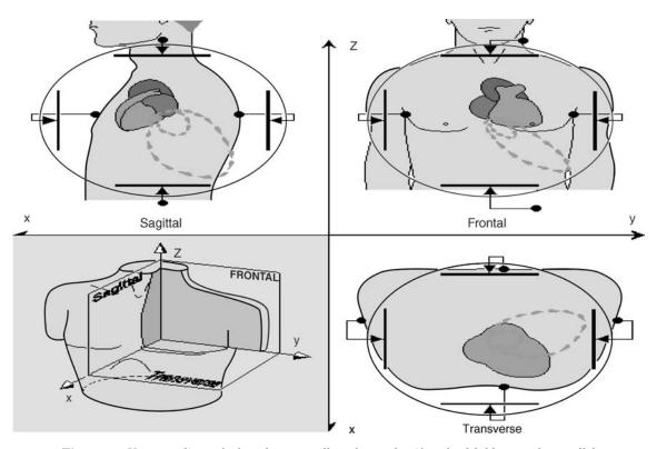
**Figure 16.** Vectorcardiography based on mutually orthogonal uniform lead fields set up by parallel electrode arrangements on opposite sides of the torso in three principal planes. (Courtesy of Ref. 2.)
