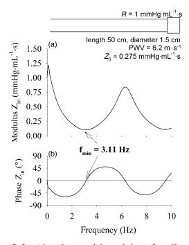
Figure 8. Input impedance modulus and phase of a uniform tube with length 50 cm, diameter 1.5 cm, characteristic impedance of 0.275 mmHg·mL<sup>-1</sup> · s (36.7 × 10<sup>6</sup> Pa·m<sup>-3</sup>·s) and wave propagation speed of 6.2 m·s<sup>-1</sup>. The tube is ended by a (linear) resistance of 1 mmHg·mL<sup>-1</sup> · s (133.3 × 10<sup>6</sup> Pa·m<sup>-3</sup>·s).
