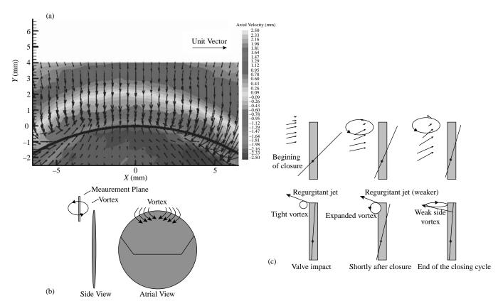
**Figure 14.** 3D phase-averaged velocity map of major orifice regurgitant flow in Bjork–Shiley monostrut valve. (a) 3 mm from valve housing, 4 ms after impact. (b) Illustration of measurement plane and vortex flow pattern. (c) Flow field schematic during valve closure determined from multicomponent LDV measurements (64).
