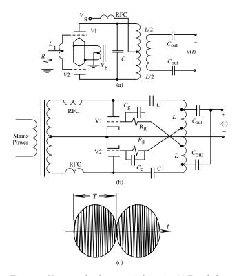
**Figure 5.** Vacuum tube electrosurgical circuits. (a) Tuned plate, tuned grid oscillator, as used in the Birtcher Electrosectilis. (b) Modified Hartley oscillator, as used in the Bovie AG. (c) Fully rectified output waveform.
