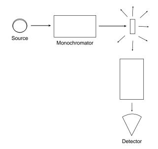
**Figure 2.** Design of a typical spectrofluorimeter. As described in the text, a desired wavelength is selected with the aid of a monochromator and is used to irradiate a sample (large arrows); light emitted by the fluorescent sample is released in all directions (small arrows). The detector is positioned at a right angle with respect to the excitation beam in order to avoid light from the exciting beam entering the detector.
