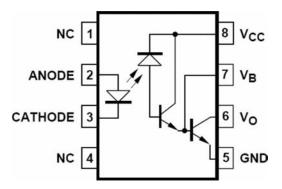
**Figure 13.** Schematic of a typical optoisolator using diode–diode coupling.
