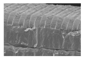
Figure 4. Microfabrication of polymer surface using a combination of reactive ion etching and compression molding. Grooves are 10  $\mu$ m wide and 3  $\mu$ m deep.
