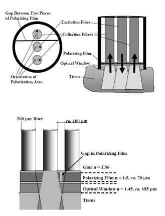
Figure 13. Design of the polarized fiber probe (62).
