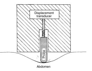
**Figure 8.** Schematic cross-sectional view of a tocodynamometer. [Reprinted with permission from CRC Press (6).]
