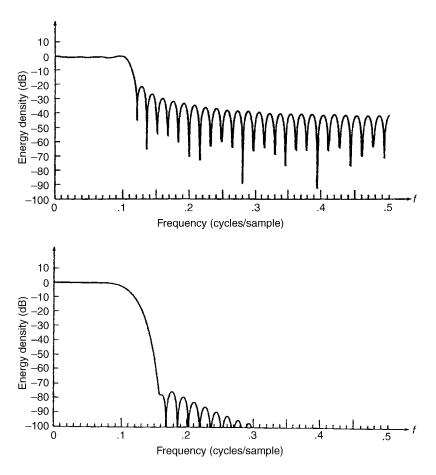
**Figure 8.** Comparison of sidelobe leakage effects in the spectrum using (a) rectangular window versus (b) Blackman window. Spectra are computed for a signal with (voltage spectrum X(f) = 1, abs(f) < 1; X(f) = 0 otherwise. The Blackman window reduces sidelobe effects and increases smoothing of the spectrum. (Adapted from Ref. 89.)
