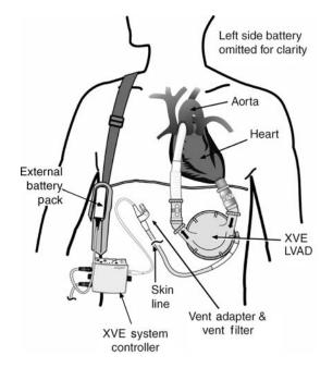
**Figure 8.** Thoratec HeartMate XVE Electric Ventricular Assist Device. The HeartMate XVE uses an electric motor and pusher plate system to pump blood. A percutaneous power line is used to connect the pump to an external battery pack and controller. (Reprinted with permission from Thoratec Corporation.)
