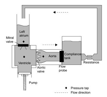
**Figure 8.** Schematic of a pulse duplicator for *in vitro* heart valve testing.
