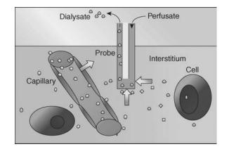
**Figure 4.** Diagram of a microdialysis probe (39). The semipermeable membrane at the probe tip allows exchange of soluble molecules between the probe and surrounding tissue. Samples are continuously collected and analyzed. (Used with permission of BMJ Publishing Group.)
