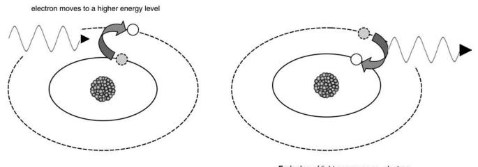
Emission of light energy as an electron moves to a lower energy level
