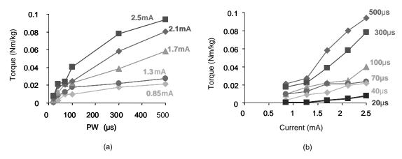
**Figure 1.** Typical force recruitment curves obtained from the ankle dorsiflexor muscle (Tibialis anterialis) of a rat through intramuscular stimulation. The recruitment curves indicate two techniques of force-torque modulation (a) pulse width modulation (PWM) and (b) pulse amplitude modulation (PAM). Single, symmetric, charge balanced, biphasic (cathodic first) pulses at an interval of 60 s were delivered. The currents were chosen as multiples of the twitch threshold current at 40 µs.
