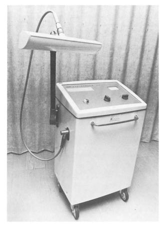
**Figure 9.** Microwave diathermy equipment. The microwave generator contains a magnetron that produces high frequency alternating current. This current is carried by a coaxial cable shown on the left to a transducer (upper left) containing an antenna and a reflector. The antenna converts the electric current into microwaves that are collected by the reflector. This focuses them and beams them into the body, where they are transduced into heat.
