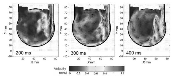
**Figure 15.** Phase-average velocity maps from mid to late diastole for a prototype artificial heart ventricular chamber (time reference is from the onset of diastole, 4.7 L·min<sup>-1</sup> CO, 75 bpm) (68).
