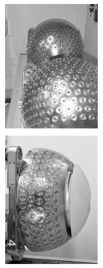
**Figure 6.** (Upper panel) Collimator helmets for Leksell Gamma Unit Model U. (Lower panel) Collimator helmet for Leksell Gamma Unit Models B and C.
