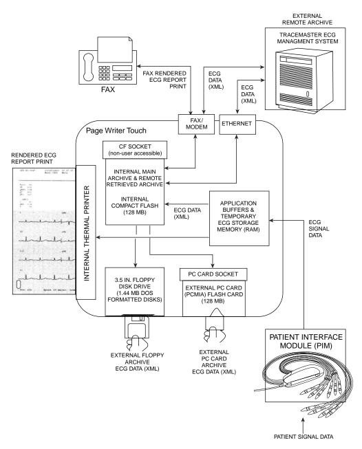
**Figure 13.** The ECG data flow and storage in PageWriter Touch electrocardiograph. (Courtesy of Philips Medical systems, USA.)
