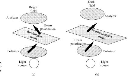
**Figure 10.** Principle of tissue birefringence. (a) Birefringent tissue is able to rotate the polarization (large arrow) of polarized light. (b) Thermally damaged tissue loses this property.
