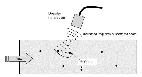
**Figure 5.** Schematic of the operation of a Doppler ultrasound probe.
