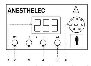
**Figure 5.** Front view of the Anesthelec generator box  $1 \rightarrow 3$  digits displayer: Current intensity (from 000 to 300 mA);  $2 \rightarrow$  Pushing button On/Off;  $3 \rightarrow$  Pushing button for increment of the output current intensity;  $4 \rightarrow$  Pushing button for decrement of the output current intensity;  $5 \rightarrow$  Pushing button to select display (intensity of voltage);  $6 \rightarrow$  Connector for the three electrodes.
