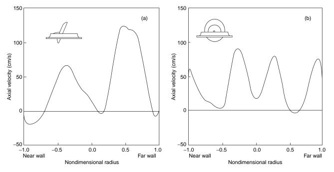
**Figure 14.** Velocity profile measured distal to a tilting disk valve in the aortic position *in vitro* in a pulse duplicator using laser Doppler anemometry technique.
