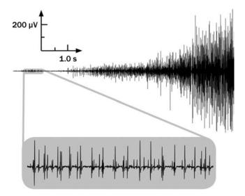
**Figure 1.** The EMG signal recorded with surface electrodes located on the skin above the first dorsal interosseous muscle in the hand. The signal increases in amplitude as the force produced by the muscle increases.
