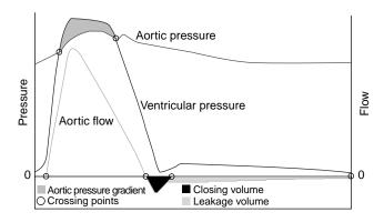
**Figure 3.** Idealized waveforms of pressure and flow through the aortic valve.
