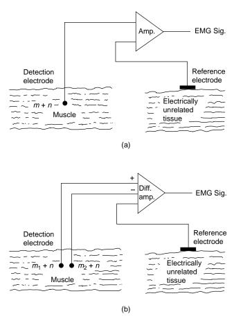
**Figure 10.** (a) Monopolar detection arrangement. (b) Bipolar detection arrangement. Note that in the bipolar detection arrangement, the EMG signals are considered to be different, whereas the noise is similar.
