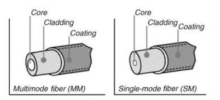
Figure 2. Types of fibers. (From Basic Principles of Fiber Optics, Corning Incorporated © 2005.)
