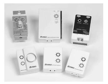
Figure 3. X-10 switching modules.
