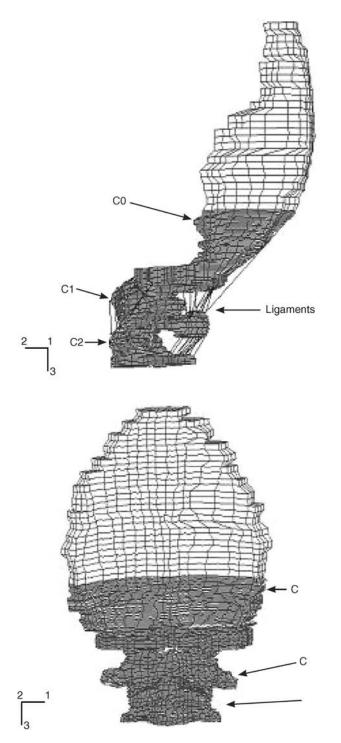
**Figure 9.** Finite element models of the upper cervical spine used to study the biomechanics of rheumatoid arthritis. (Taken from Ref. 66.)
