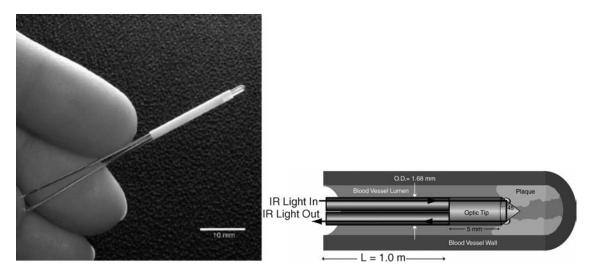
**Figure 3.** An example of a HWG endoscope. Both diagnostic and therapeutic applications have been demonstrated by coupling a high refractive-index conic tip (sapphire and zinc sulfide) to a HWG. In this geometry with two waveguides, diagnostic spectrometer light can be coupled into the tip in contact with tissue via one waveguide and sent back to a detector via the other waveguide.
