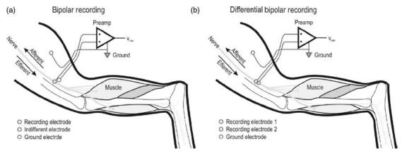
**Figure 8.** Bipolar recording configurations. (a) Shows a standard bipolar configuration where the signals from one recording electrode are amplified with respect to a second electrode that samples the ambient noise, the indifferent electrode. A separate ground electrode is placed somewhere in the tissue. The differential bipolar recording configuration (b) places a second recording electrode in or on the nerve and the difference of the signals from two active electrodes is amplified.
