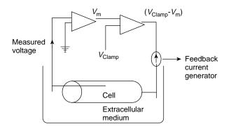
**Figure 1.** Simplified circuit representation of a voltage-clamp setup (8).
