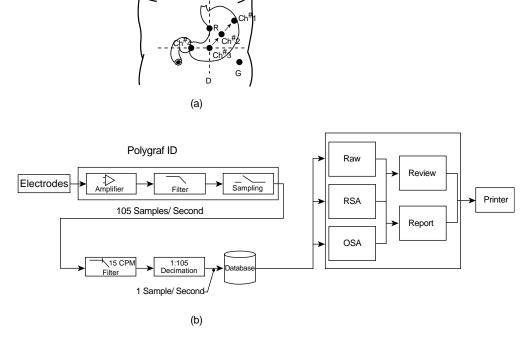
**Figure 5.** (a) Electrogastrogram electrodes placement for making four-channel EGG recordings consists of placing four active electrodes along the antral axis of the stomach, a reference electrode over the xyphoid process, and a ground electrode on the patient's left side. (b) Block diagram of Medtronic POLYGRAM NETTM ElectroGastroGraphy System (RSA: Running Spectral Analysis; OSA: Overall Spectral Analysis). (Reprinted with permission of Medtronic, Inc.).
