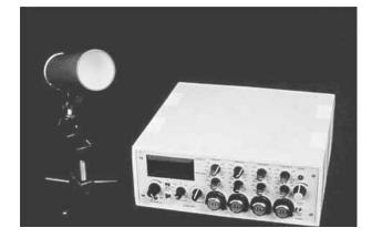
Figure 3. A "mini-Ganzfeld" based on light emitting diode technology. The device shown has four independent color channels, blue, green, orange and red, each of which can be used as stimulus or background alone or in combination. (Courtesy of Chris Hogg, CH electronics, Bromley, Kent, UK; www.ch-electronics.net.)
