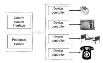
Figure 1. Components of an EADL system.
