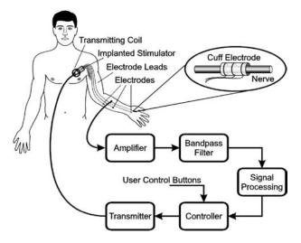
**Figure 27.** A neural prosthetic system for lateral-key grip restoration after spinal cord injury including sensory feedback. The FreeHand stimulation system (developed at Case Western Reserve University, Ohio) was modified to take advantage of natural sensory feedback signals obtained from a cutaneous, digital nerve in the hand. (Adapted from Ref. 92 with permission.)
