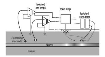
**Figure 14.** Use of optoisolated amplifiers and an optoisolated stimulator eliminates the ground loops shown in Fig. 8 by eliminating low impedance return paths to the tissue or stimulator circuit. Note that each isolated subcircuit has its own independent ground. Moreover, since there is no current flowing through the main ground from the tissue (shown as a dashed triangle), the main ground does not need to be grounded to the tissue.
