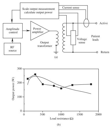
with fixed output impedance 300  $\Omega$  and maximum output power of 250 W at 300  $\Omega$  load impedance. The differences at high load impedances typical of electrosurgical cutting (up to  $\sim 2~k\Omega$ ) are easily seen in the figure.
