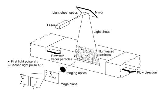
Figure 16. Schematic of a PIV setup (66). (With kind permission of Springer Science and Business Media.)
