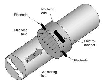
**Figure 2.** Illustration of the principle of operation of the electromagnetic flow meter. Note, the magnetic field, electrodes, and flow direction are all mutually perpendicular to one another.
