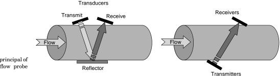
**Figure 3.** Illustration of principal of transit time ultrasonic flow probe operation.
