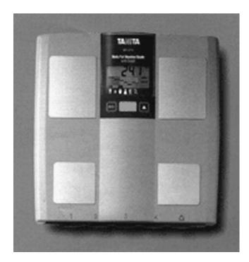
**Figure 11.** A scale with bioelectrical impedance analysis. This is a simple version of body impedance analysis using leg-to-leg bioimpedance analysis. The precision electronic scale has two footpad electrodes incorporated into its platform. The measurement is taken while the subject's bare feet are on the electrodes. The body fat percentage can be obtained from equations based on weight, height, and gender.
