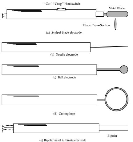
**Figure 1.** Electrodes typically used for general electrosurgery.
