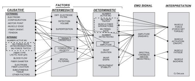
**Figure 2.** Relationship among the various factors that affect the EMG signal. [Reproduced with Permission from C. J. De Luca, "The Use of Surface Electromyography in Biomechanics." In the Journal of Applied Biomechanics, Vol. 13(No 2): p 139, Fig. 1.]
