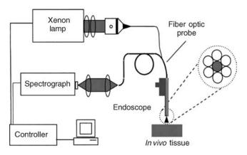
Figure 12. Schematic diagram of the LSS system (59).
