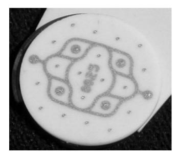
**Figure 11.** Close-up view of tissue glucose and oxygen sensor array (77). Sensor array with small ( $125 \,\mu$ m diameter) independent platinum working electrodes, large ( $875 \,\mu$ m diameter) common platinum counterelectrodes, and a curved common Ag/AgCl reference electrode. The membrane is not present. (Copyright 2003, American Physiological Society.)
