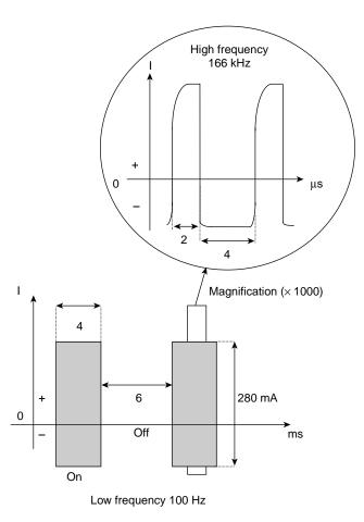
**Figure 2.** The Limoge waveform pattern: a modulated HF (166 kHz) pulse trains (top) regularly interrupted with a repetition cycle of 100 Hz. Concerning the high frequency, note the exponential ascent and acute fall of the waveform, and also note the area of the positive deflection is equal to that of negative deflection.
