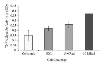
**Figure 2.** TNF- $\alpha$  release (specific activity  $\pm$  95% confidence limits) as a result of challenge with UHMWPE particles, which were noncross-linked (NXL), cross-linked with 5 Mrad of irradiation, cross-linked with 10 Mrad of irradiation compared to the cell only control.
