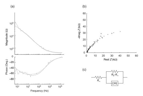
**Figure 15.** (a) Shows a typical metal electrode impedance spectrum and its fit to the Cole model shown in (c). (b) is the Warburg representation of the impedance spectrum where the real Z is plotted with respect to the negative of the imaginary Z.
