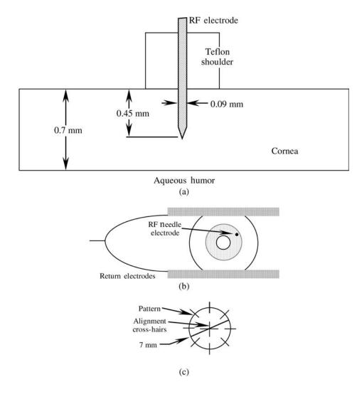
**Figure 15.** Needle electrode used to shrink corneal collagen and change curvature for correction of hyperopia. (a) Cross-section of electrode in place, (b) View of speculum return electrodes, (c) spot pattern for shrinkage lesion location. [Reproduced with permission from "Corneal reshaping by radio frequency current: numerical model studies" Proc. SPIE v4247 (2001) pp109–118.]
