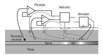
**Figure 12.** Illustrates potential ground loop currents that can be induced during stimulation if multiple ground electrodes (shown as triangles) are used. Since each ground electrode represents the same potential, the nearest ground electrode can draw current, which passes through the ground plane and out of the other ground electrodes, increasing the uncertainty of the point of stimulation.
