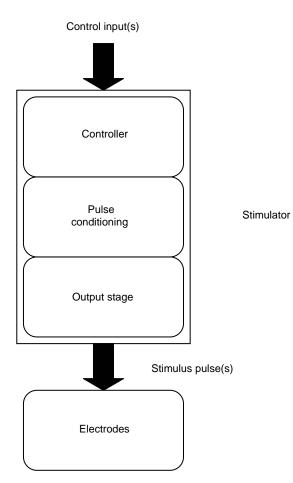
**Figure 2.** The FES systems typically incorporate control signals from the user that a Controller stage acts upon. Patterns of stimulation pulses are shaped with a pulse conditioning module that in turn feeds pulse information to an output stage that delivers regulated-current or regulated-voltage pulses of the desired amplitudes and timing to one or more channels of electrodes which are in contact with, or implanted within, the body.
