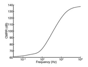
**Figure 17.** The frequency dependence of the CMRR is shown for an ideal preamplifier using electrodes that are mismatched by 10%. The frequency dependence of the electrodes has a large influence in the CMRR, which resembles the inverse of the electrode impedance.
