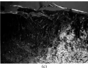
**Figure 11.** Disk electrode applied to myocardium. (a) Geometry. (b) Light microscopic view of region in dashed rectangle at the edge of the electrode. Original magnification  $40\times$ . (c) Transmission Polarizing Microscopy (TPM) view of the same section showing the clear delineation of the zone of birefringence loss. Original magnification  $40\times$ .
