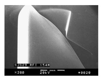
**Figure 6.** Detail of the St. Jude Medical bileaflet valve pivot mechanism. A tab on the leaflet inserts into a butterfly shaped depression in the valve annulus ring. The pivot depression retains and guides the leaflet motion during opening and closing excusions.
