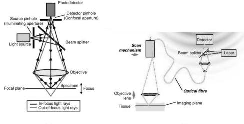
**Figure 9.** Confocal microscopy. (a) Principle of confocal arrangement. (From MPE Tutorial, Coherent Incorporated © 2000.) (b) Possible implementation of fiber-based confocal microscope (36).
