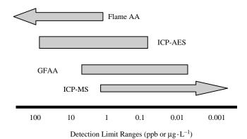
**Figure 5.** Typical detection limit ranges for major spectrometry techniques. Flame atomic absorption, inductively coupled plasma-atomic emission spectrometry, graphite furnace atomic absorption, inductively coupled plasma-mass spectrometry (19).
