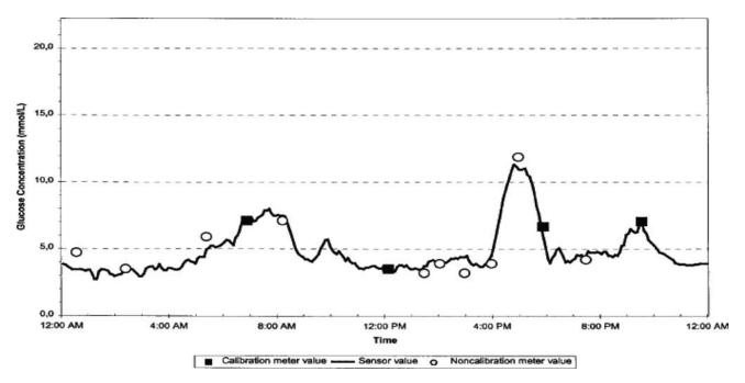
**Figure 8.** An example of the CGMS sensor response (65). Squares are reference values utilized in sensor calibration. Circles are additional reference blood glucose values. Reference values were obtained from a standard glucose meter. Values are in mmol·L<sup>-1</sup>. (Used with permission.)
