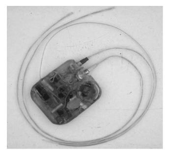
**Figure 9.** Animal prototype long-term central venous glucose sensor with implanted telemetry (73). Glucose and oxygen sensors are at the end of the catheters. Telemetry antenna emerges from the top, left. The telemetry body is  $2 \times 2.5$  in.
