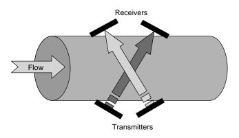
Figure 4. Bidirectional wave propagation.
