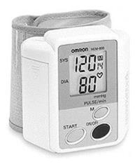
**Figure 4.** Wrist-type home blood pressure monitor. The measurement site is the wrist and during the measurement, the wrist must be at heart level.
