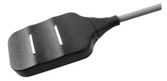
**Figure 6.** Examples of active surface electrode in bipolar configurations from Delsys Inc. The spacing between the bars is 10 mm, the length of the bars is 10 mm and the thickness is 1 mm. These electrodes do not require any skin preparation or conductive paste or gels.
