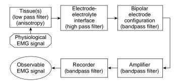
**Figure 9.** Block diagram of all the major aspects of the signal acquisition procedure. Note the variety of physical properties that act as filters to the EMG signal before it can be observed. The term "physiological EMG signal" refers to the collection of signals that emanate from the surface of the muscle fibers. These are not observable.
