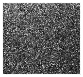
Figure 19. Example of a PIV particle image.
