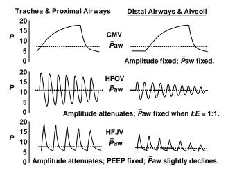
Figure 11. HFV Airway Pressure Waveform Dampening. (Used with permission. © 2003, Bunnell Inc.)
