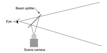
Figure 13. Use of a beam splitter to minimize scene camera parallax.
