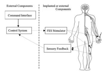
**Figure 25.** Illustration of the basic elements in a closed-loop neuroprosthesis application. The instrumentation typically includes an external (i.e., outside of the body) command interface and control system and external/implanted interfaces for sensing or activating the biological tissue.
