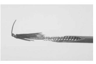
Figure 7. A "Peterson" type intramuscular electrode design. This is a helically wound PFS insulated multistranded 316LVM stainless steel wire design that is attached to a barb-like anchoring structure constructed of polypropylene suture material. The wound section of the electrode is  $\sim 800\,\mu m$  in diameter and is partially loaded into a hypodermic needle. (Courtesy of J.T. Mortimer and reproduced by permission of World Scientific Publishing Co.)
