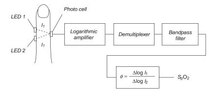
**Figure 17.** The principle of the oximeter. Hemoglobin absorbs light and the amount depends on whether it is saturated with oxygen. The absorption at two wavelengths (650 and 805 nm) is measured and used to calculate the proportion of hemoglobin that is oxygenated.
