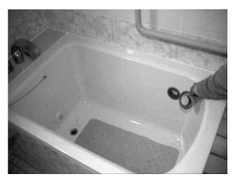
**Figure 7.** The ECG recorded from a bathtub. Silver–silver chloride electrodes are placed in the bathtub and the ECG signal can be obtained though the water.
