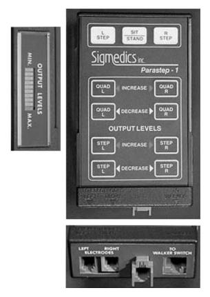
**Figure 5.** The neuromuscular stimulation unit for the Parastep system manufactured by Sigmedics, Inc. is battery-powered and microcomputer controlled. Cables connect the unit to surface electrodes, as well as to finger activated control switches on a walker. (Courtesy of Sigmedics, Inc.)
