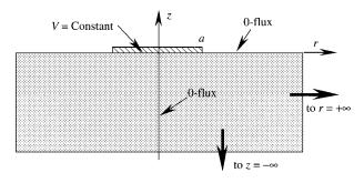
**Figure 23.** Solution geometry for disk electrode applied to infinite medium. Return electrode, V=0, located at  $r = \infty$  and  $z = -\infty$ .
