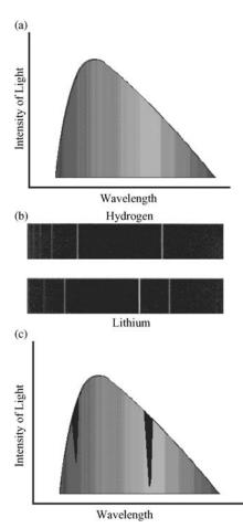
**Figure 1.** Emission and absorption spectra: (a) A continuous spectrum emitted from a hot solid, liquid, or gas under pressure. (b) A line spectrum emitted from a low pressure hot gas. (c) A dark line or absorption spectrum observed when a continuous spectrum is viewed behind a cool gas at low pressure.
