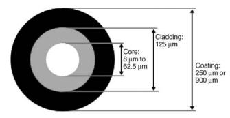
Figure 3. Fiber components. (From Basic Principles of Fiber Optics, Corning Incorporated © 2005.)
