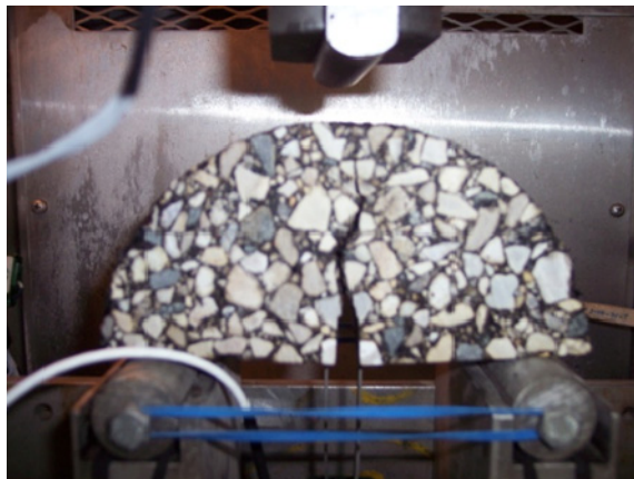
Fig. 1. Semi-circular beam fracture test setup
