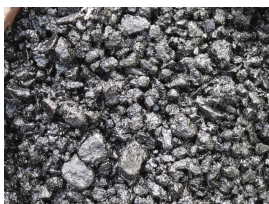
Fig. 2. Mixture of 50%RA with virgin aggregate without adding virgin bitumen
