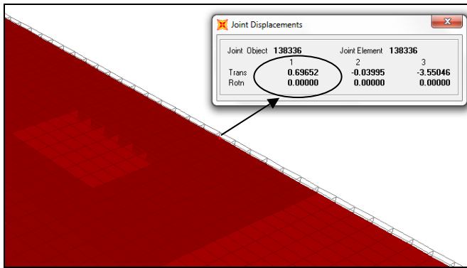
Fig. 11. Lateral displacement of the pavement (0.697mm)
