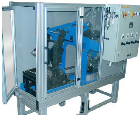
Fig. 2. University of Canterbury roller compactor used to prepare AC10 and AC14 fatigue beams
