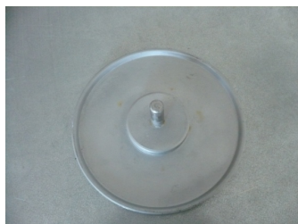
Fig. 1. Equipment used to trowel the slabs
