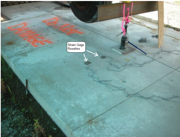
Fig. 3. Bottle jack positioned at center-edge of slab
