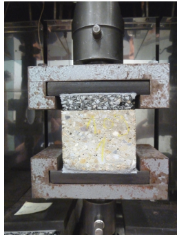
Fig. 6. Cubical specimen clamped in the pulling device - BRRC direct tensile test method
