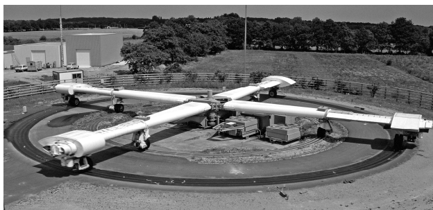
Fig. 1. The pavement fatigue carousel of IFSTTAR
