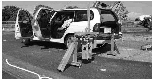
Fig. 6. Picture of motorised bench with two ETSA over the pavement
