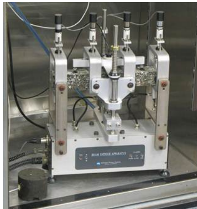
Fig. 3. University of Canterbury bending beam fatigue apparatus
