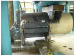
Fig. 5. Cylinder Dir Shear Test
