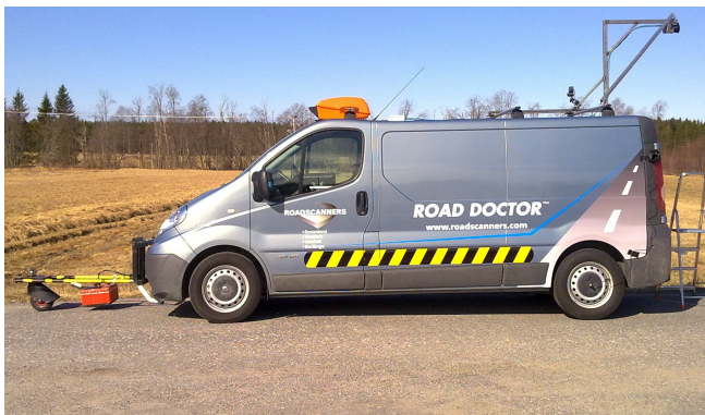
Fig. 1. A survey van equipped with GPR, thermal cameras and laser scanner.
