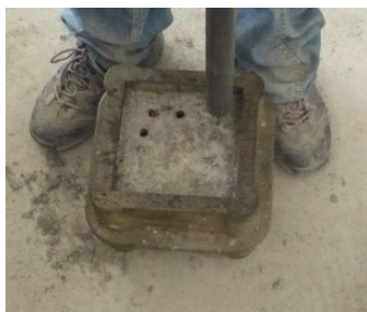
Fig. 3. Needle to measure the resistance to penetration
