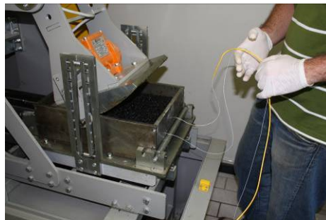
Fig. 3. Compaction of the second layer of bituminous concrete
