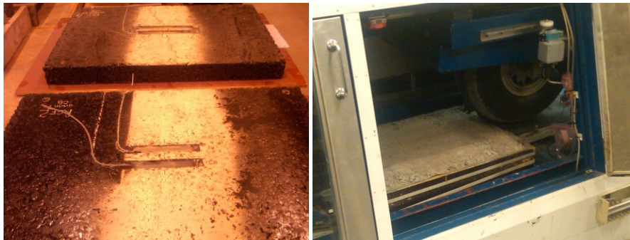
Fig. 4. (a) Strain gauges instrumentation; (b) WTT equipment
