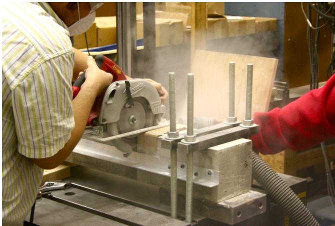
Fig. 2. Saw cutting of cantilever concrete beam
