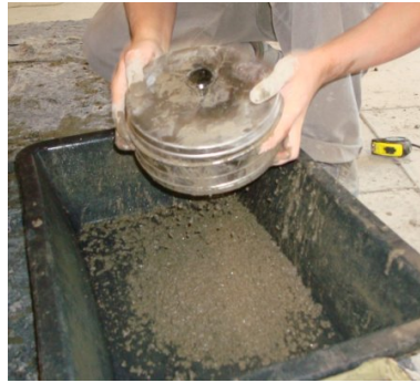
Fig. 4. Sieving of the concrete
