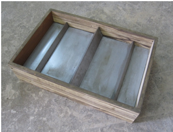
Fig. 2. Plywood mold with the stress risers
