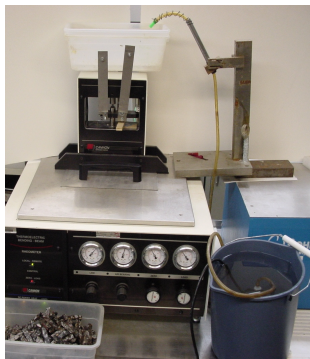
Fig. 1. Bending Beam Strength (BBS) apparatus
