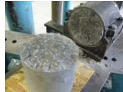
Fig. 6. Failed Section (PMC2)
