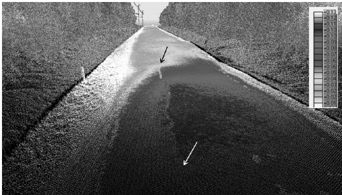
Fig. 8. An example frost heave view of laser scanner point cloud data.
