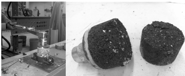
Fig. 7. Torque Bond Test laboratory setup and failed specimen
