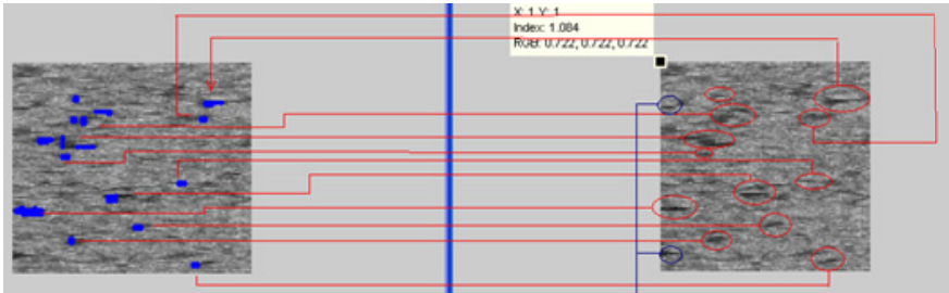
Fig. 9. Example of the automatic detection of aggregate loss in range images
