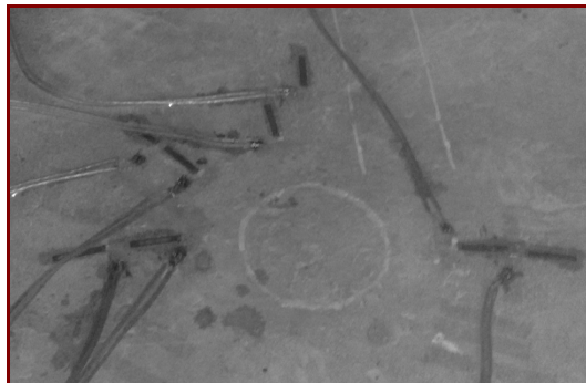
Fig. 6. Positions of strain gages and core-ring drilling
