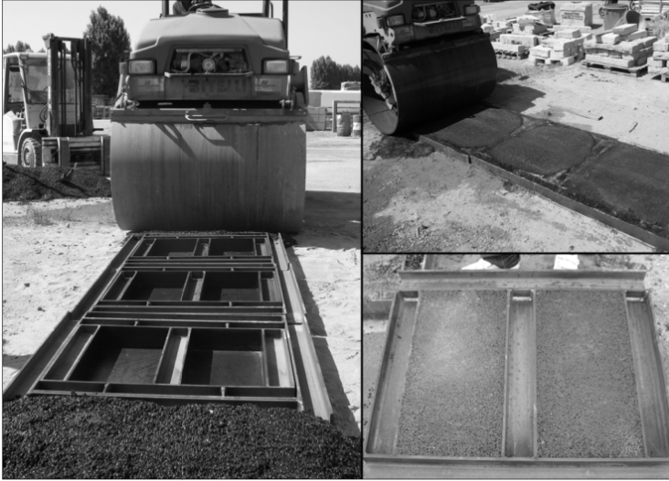
Fig. 2. Field compaction with specific mold
