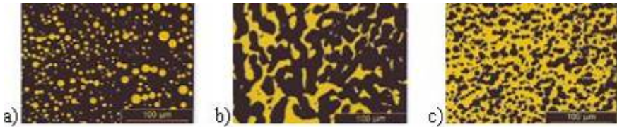
Fig. 1. Microstructure of bitumen / polymer blends: a) Continuous bitumen phase b) Bitumen with inter-twisted phases c) Continuous polymer phase (AIPCR) [3]
