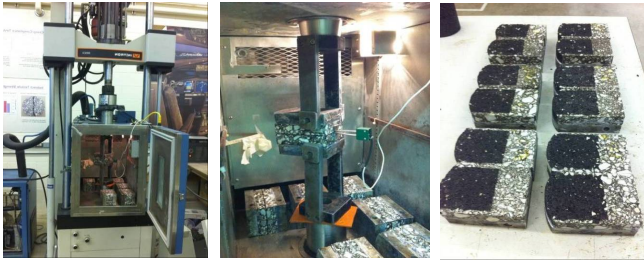
Fig. 5. IBT test setup and failed specimens
