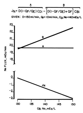
Figure 1. Effect of diffusive Na gradients on net Na flux  $(J_N)$  at fixed  $Q_F = 10$  ml/min.
