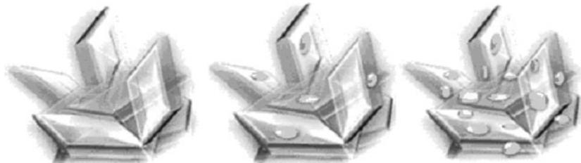
FIGURE 23.3 Accumulation of biological materials changes the resonant frequency of a piezoelectric crystal.
