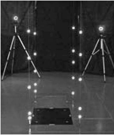
FIGURE 6.6 The X , Y , Z coordinates of the control points (i.e., reflective targets) are known relative to the origin of the object-space. Once the cameras have been calibrated, the hanging strings with the control points are removed from the field of view of the cameras. The black rectangle flush with the floor is a force platform (see Sec. 6.4.5).
