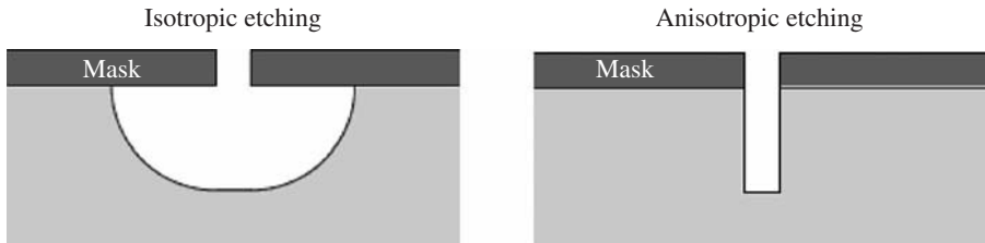
FIGURE 24.4 Isotropic and anisotropic etching.
