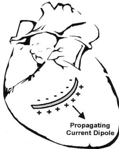
FIGURE 20.16 Illustration showing the simplified concept of a traveling band of depolarization creating a net current dipole in the heart.
