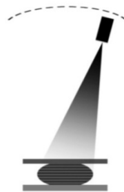
Fig. 1. X-ray tube rotates in an arc 15° or 30° above the breast
