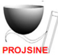
Fig. 1. Image illustrating the projected sine-wave (PROJSINE) 3D trajectory used in acquisitions. The PROJSINE orbit allows for nearly-complete sampling of the breast volume while providing useful data from the chest wall that may otherwise not be collected.
