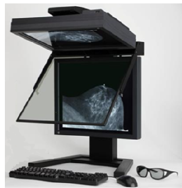
Fig. 2. 3D display consisting of 5 mega pixel grayscale monitors with a half mirror
