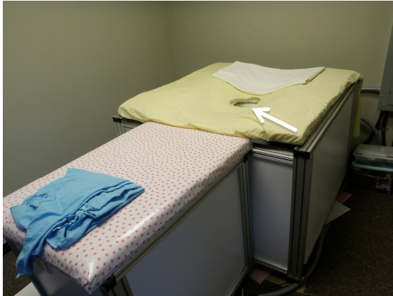
Fig. 1. Completely shielded breast CT system enclosure used for imaging. Upper right section covered in a yellow sheet is where the patient lies prone and extends her breast through the opening (white arrow). Lower left section covered in pink polka-dots is for hip and leg support. The inside of this section is also used for housing various motion control components.
