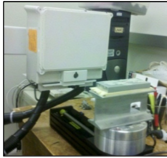
Fig. 1. Gamma camera (top left) and vertical axis rotation stage (lower right), mounted atop the linear translation stage. For clarity the phantom is not shown.
