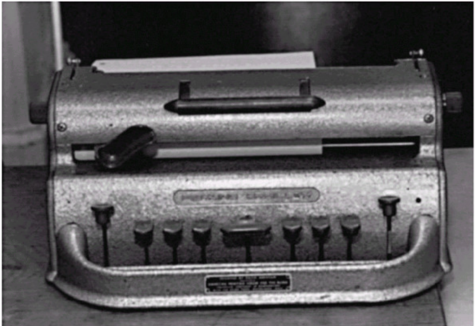
Figure 28.1 A Braille writer. Any combination of the six keys is pressed simultaneously to make one Braille letter, number, or symbol.
