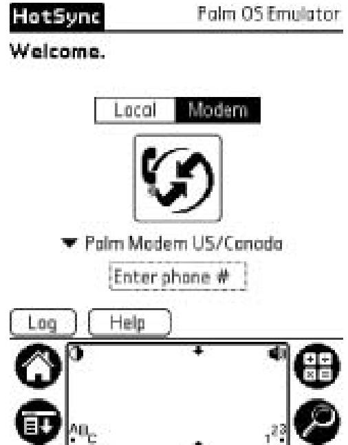
FIGURE 15.24. To connect to a LAN or PC via a modem or cellular phone, select “Modem” in the opening “HotSync” screen and the appropriate modem you will be using. Then tap on “Enter phone #” to plug in the number you will be calling. Now tap on the icon with the “HotSync” symbol in the center of the screen to start the synchronization. (Reprinted with permission from palmOne, Inc.)
