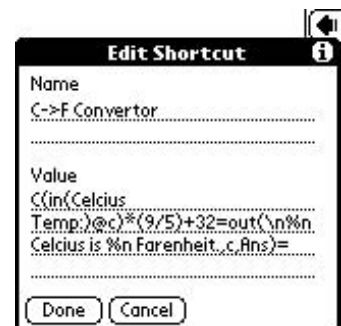
FIGURE 16.7. Shortcut code for temperature conversion. (Reprinted with permission from Installigent Team, a Zero-sixty Corp.)
