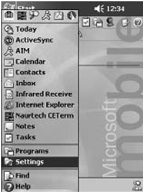
FIGURE 15.25. Tap on the Start menu in the upper-left-hand corner, then select “Settings.” (Reprinted with permission from Microsoft Corporation.)
