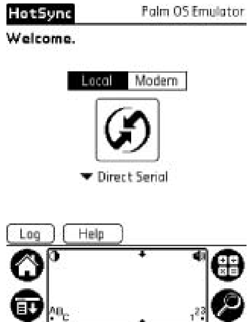
FIGURE 15.22. Next, select the drop-down menu next to “Direct Serial” for synchronization via infrared (IrDA). If you have a wireless LAN driver installed, it will appear here as well. (Reprinted with permission from palmOne, Inc.)
