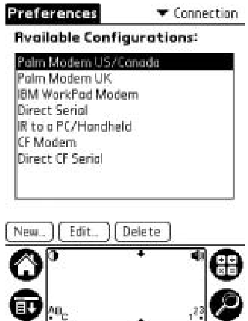
FIGURE 15.8. Fourth, select the appropriate type of modem. If you are connecting via a cellular phone, first try the “Palm Modem” for your region. Then tap on the button at the bottom labeled “Edit.” (Reprinted with permission from palmOne, Inc.)
