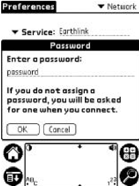
FIGURE 15.15. Enter password now or leave blank to be asked once connected. As you can see, the password appears in plain text, so you might not want to store it here. Then tap on “OK.” (Reprinted with permission from palmOne, Inc.)
