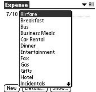
FIGURE 2.10. Example of program using pop-up menus for text entry. (Reprinted with permission from palmOne, Inc.)
