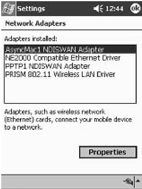
FIGURE 15.33. Find the Adapter that you will be using. Again, if you have the drivers installed correctly, it should appear in this window. Then tap on “Properties.” The next screen will prompt you for specific information for configuring the card with information such as using a server-assigned IP address versus a specific IP address, and options for named servers as well. If connecting to a network, check with the administrator for these settings. If doing this at home, try the server-assigned default and keep your fingers crossed. The network settings can drive you nuts, and my experience has been that trial and error ends up being the best way to determine the best settings due to variations in computer and network settings. (Reprinted with permission from Microsoft Corporation.)
