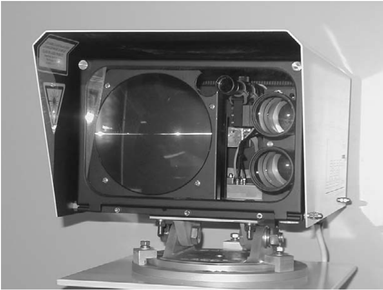
Figure 8.1 An over-the-air (atmospheric) optical communications system. It can accommodate a range of information. (Courtesy of ICS, Inc.)
