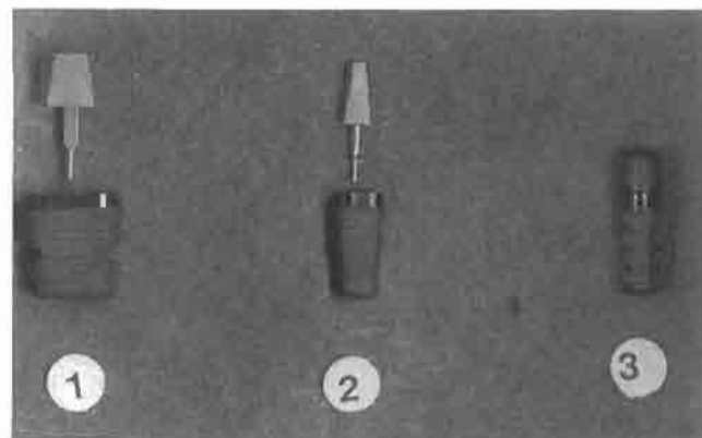
FIG. 8. Examples of carbon and carbon-silicon endosteal root form implants. (1) and (2) Vitredent (C), two-stage. (3) Carbomedics (C-Si), one-stage.
