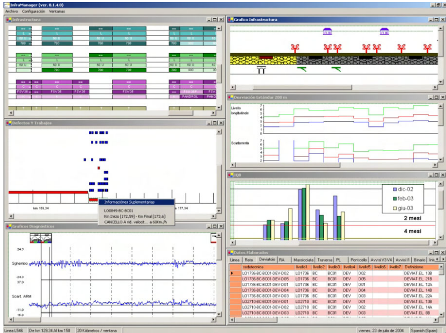
Fig. 8. Graphical diagnostics and technical condition analysis of the railway transportation infrastructure in Ramsys DSS
