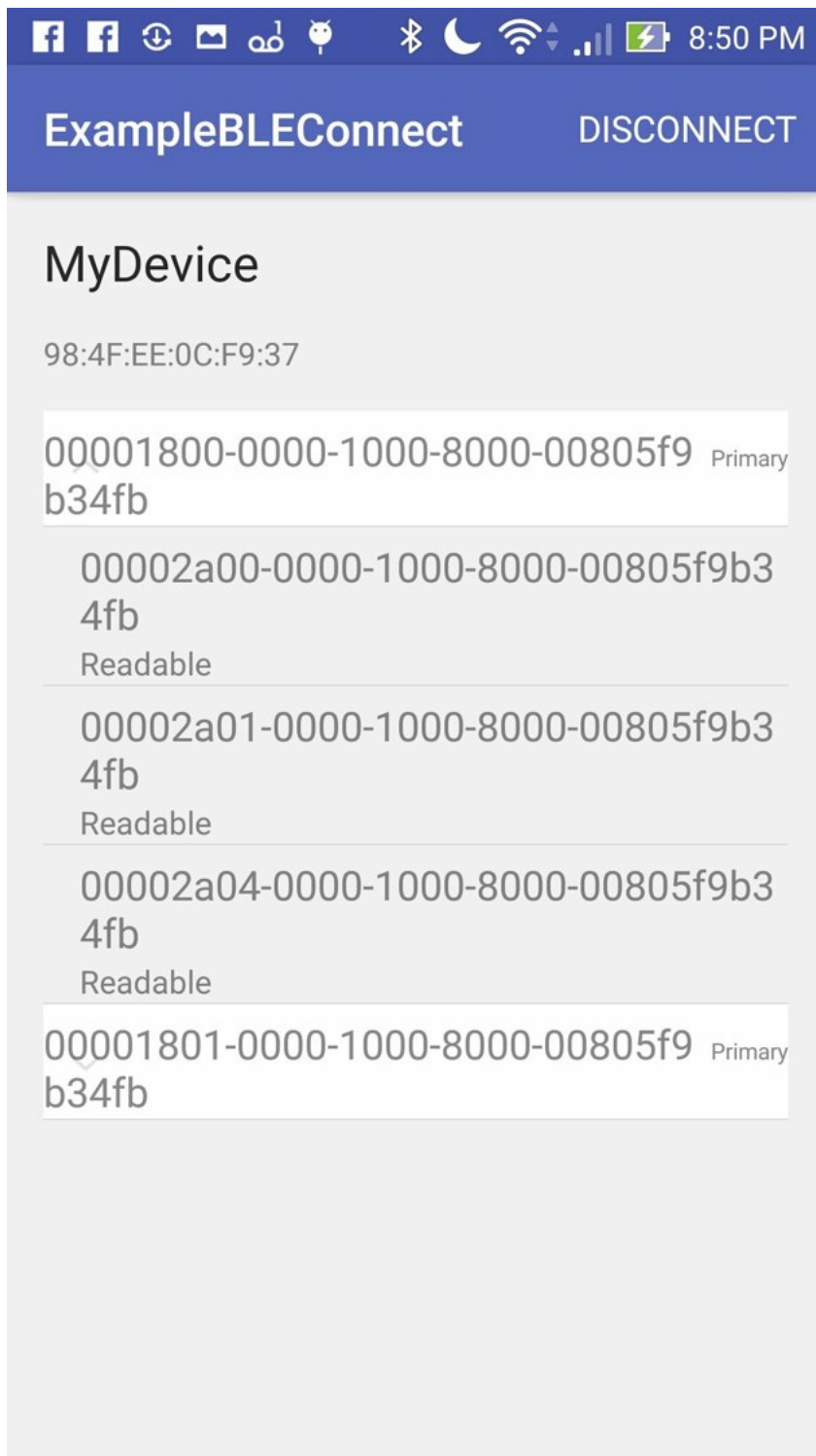
Figure 4-2. Android app shows GATT Profile of a connected Peripheral
