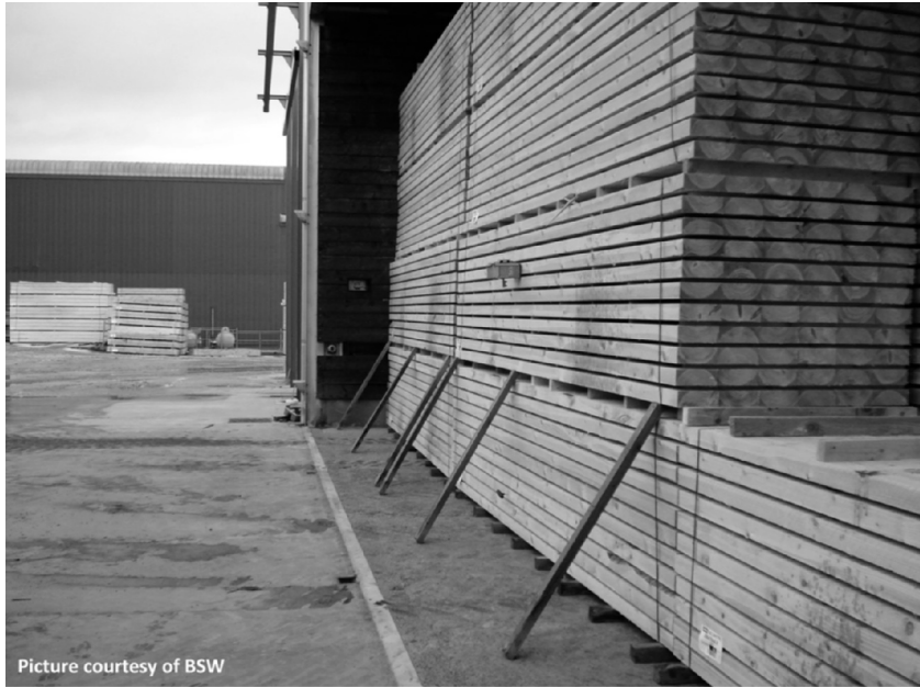
Figure 3.3b Timber correctly stacked and awaiting drying in a kiln (photo courtesy of BSW Timber plc)
