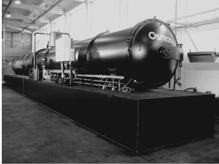
Figure 7.2 A typical high pressure treatment tank (photo courtesy of Osmose)
