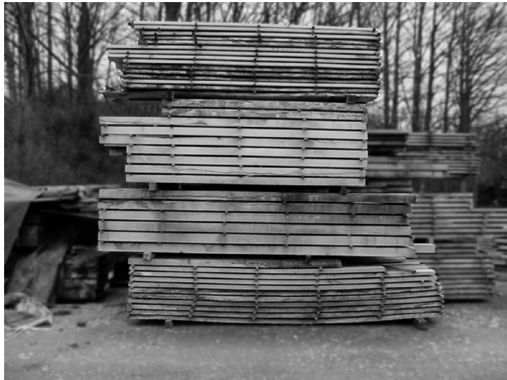
Figure 3.4 Timber stacked for air drying – but not very well !
