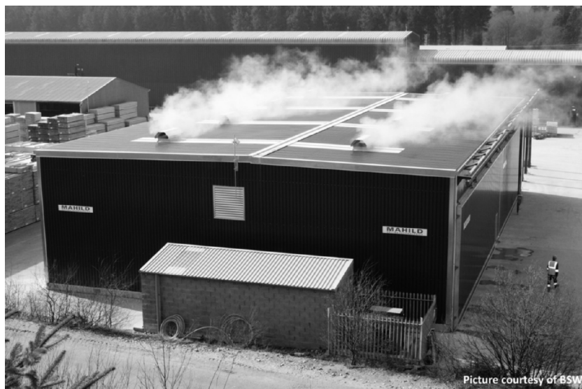
Figure 3.3a A typical drying kiln (photo courtesy of BSW Timber plc)
