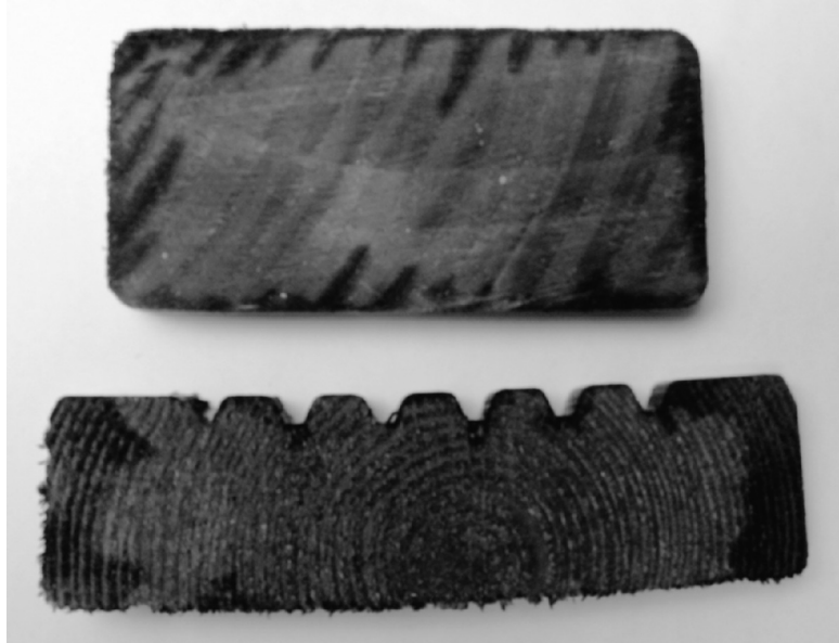
Figure 7.1 Treated zones in spruce (upper) and pine (lower). Note the low penetration into the pine heartwood
