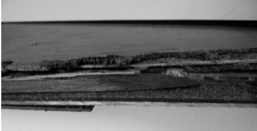
Figure 10.3 Delaminated veneers in a tropical hardwood plywood
