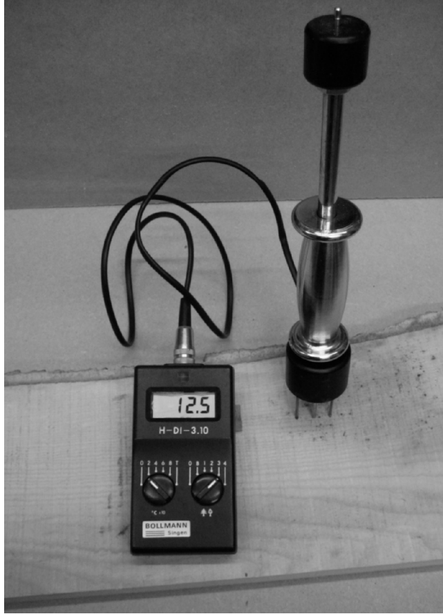
Figure 3.1 Electrical resistance-type moisture meter with hammer probe
