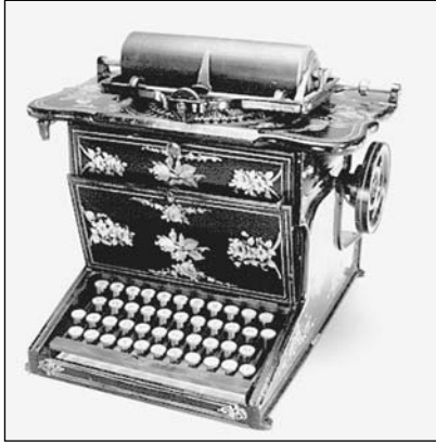
Figure 39. The Sholes and Glidden typewriter, the world's first commercially successful typewriter
