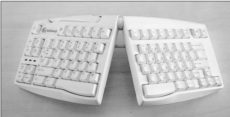
Figure 22. The adjustable keyboard is suitable for daily use as well as training. Note the split spacebar.
