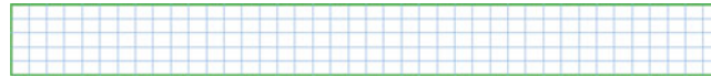
Fig. 8.8 Finite element model of tension, compression or fatigue specimens after thermal cycling or UV. Only the gauge length was modeled
