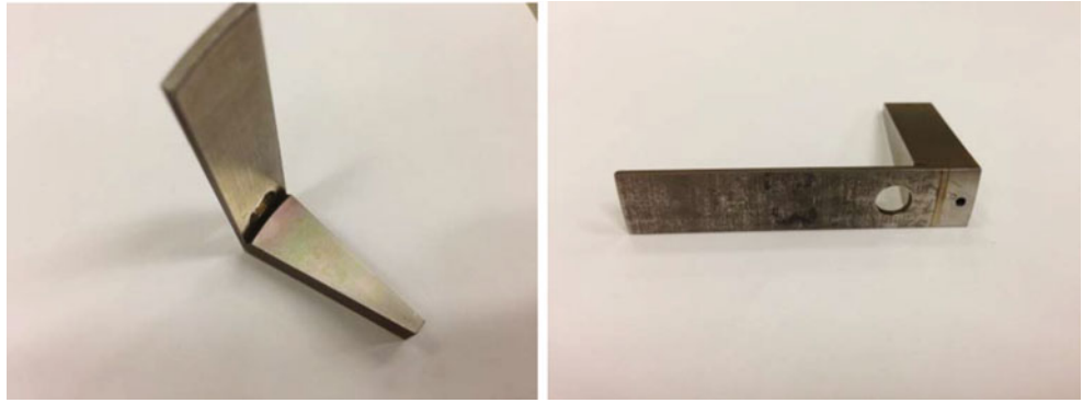
Fig. 2.3 Photographs of wedge specimens after removal from can structure
