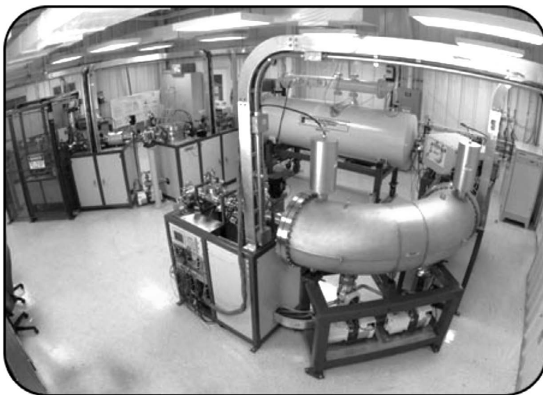
FIGURE 17.1 1 MV accelerator mass spectrometer at the Lawrence Livermore National Laboratory (LLNL). (From http://bioams.llnl.gov/equipment.php .)
