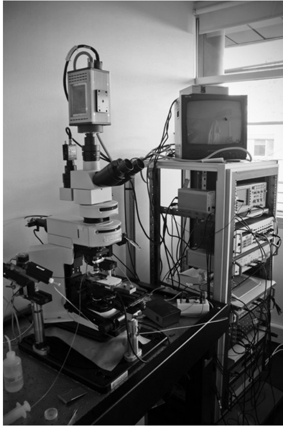
Fig. 2. Picture of an electrophysiological set-up.
