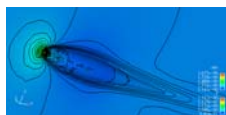
Fig. 11 Laminar BTC0 test case: the pressure is displayed in color, the density with isolines
