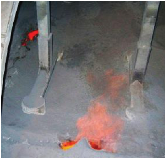
FIGURE 2.1 Anode cover material overflowing the anode yokes and collapsing due to its high internal temperature exceeding the phase change temperature of the crust.
