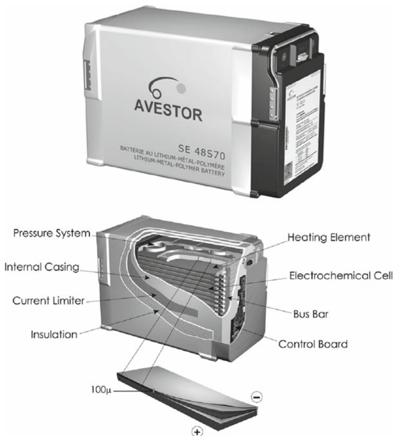
Fig. 21.3 Outlook and internal structure of the lithium pure polymer battery that Avestor has commercialized
