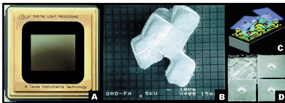
Fig. 4.1 DMD structure. (A) Texas Instruments Digital Micromirror Device. (B) Photomicrograph of a section of the micromirror array, with a grain of table salt shown for comparison. Each mirror is 16 \mu\text{m} square, on a 17 \mu\text{m} pitch. (C) Diagram of two micromirrors, with one mir-
