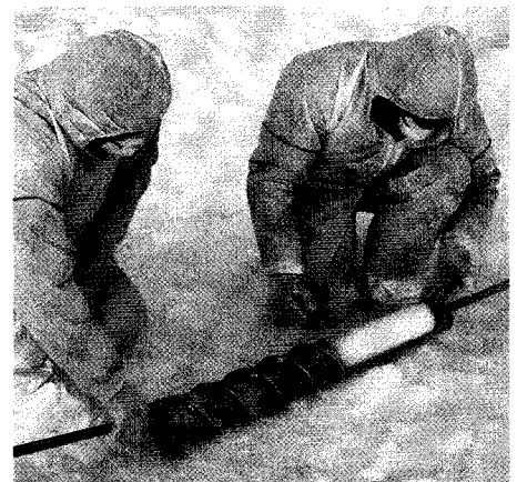
Figure 4.7 Ice core. By analyzing ice cores, scientists can measure the concentration of carbon dioxide that was present in early atmospheres.
