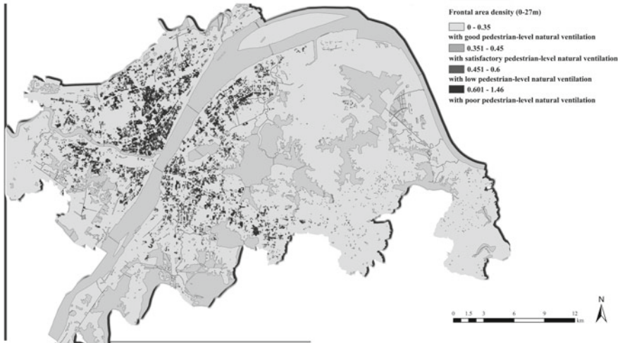
Fig. 3.3 Urban permeability map of the pedestrian-level natural ventilation in Wuhan (For interpretation of the references to color in the text, the reader is referred to the electronic version of this book)
