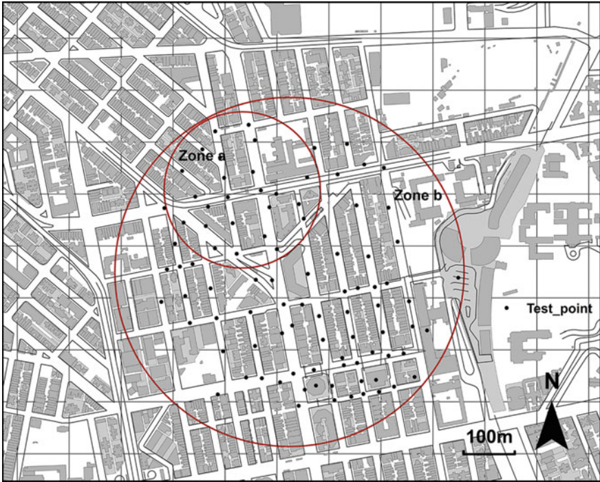
Fig. 4.5 Test points in test locations (Mong Kok as the example). Every test location includes two zones (Zone a and Zone b)
