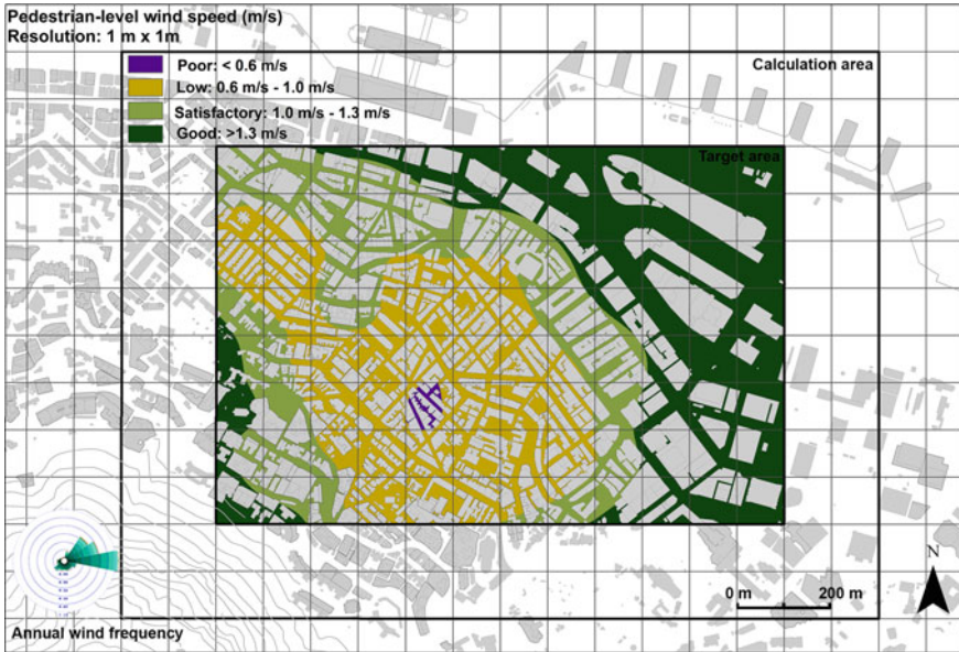
Fig. 4.11 Pedestrian-level wind speed map, which was classified as Class 1 (Poor, <0.6 m/s), Class 2 (Low, 0.6–1.0 m/s), Class 3 (Satisfactory, 1.0–1.3 m/s), and Class 4 (Good, >1.3 m/s) (For interpretation of the references to color in the text, the reader is referred to the electronic version of this book)
