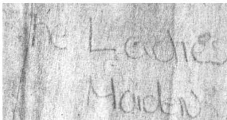
Figure 18.21 Electrostatic image of indentations from handwritten entry on previous page of an appointment calendar.
