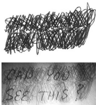
Figure 18.19 Reflected infrared (bottom) and infrared luminescence examinations can reveal otherwise illegible obliterations (top).
