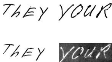
Figure 18.17 Examples of ink reactions under reflected infrared light (they — upper normal light, lower infrared reflected) and infrared luminescence (Your — upper normal light, lower infrared luminescence). Ink can also virtually disappear under such examinations. Differences in these reactions are evidence of different inks.
