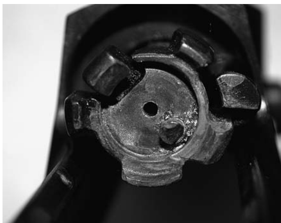
Figure 16.9 The bolt (breech) face supports the head of the cartridge during firing. The extractor is located in the upper left, the ejector in the lower right, and the firing pin aperture in the center of the bolt face.
