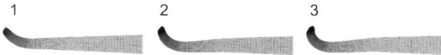
Figure 5 - Progression of three impacts by a 1000 micron particle at a velocity of 454 meters per second. Note that a majority of the vertical deformation occurs after the initial impact.
