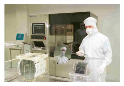
Fig. 6.9 Processing of the silicon wafers with 30 cm diameter. (photo Wacker Chemie AG)
