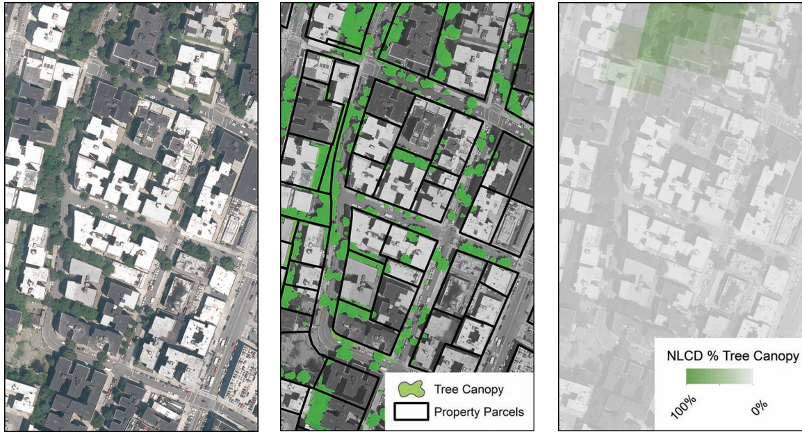
Plate 2. Comparison of land cover classifications derived from high-resolution National Agricultural Imagery Program (NAIP) imagery and mid-resolution Landsat TM imagery of the same area. (a) High-resolution imagery for an area in New York City; (b) classifies those portions of the area with tree canopy cover, using the NAIP imagery; (c) classifies the same area using the Landsat TM data (National Landcover Database). Comparing (b) and (c) shows that Landsat TM data are insufficient for detecting fine-scale vegetation in the more heterogeneous parts of the study area.
