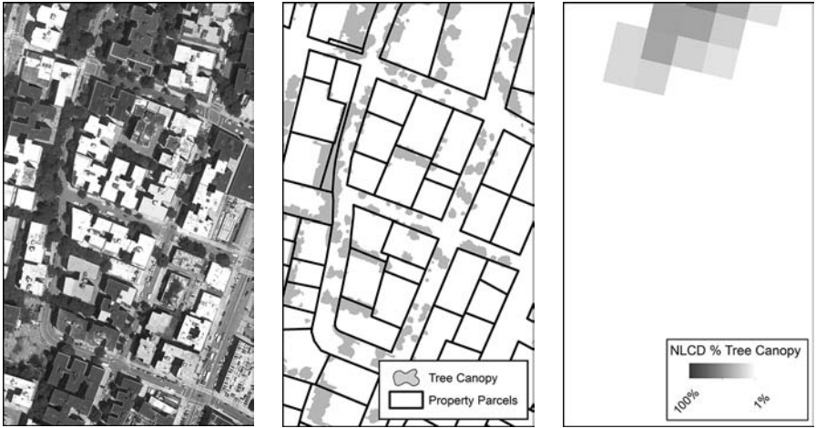
Figure 5.1. Comparison of land cover classifications derived from high-resolution National Agricultural Imagery Program (NAIP) imagery and mid-resolution Landsat TM imagery of the same area. (a) High-resolution imagery for an area in New York City; (b) classifies those portions of the area with tree canopy cover, using the NAIP imagery; (c) classifies the same area using the Landsat TM data (National Landcover Database). Comparing (b) and (c) shows that Landsat TM data are insufficient for detecting fine-scale vegetation in the more heterogeneous parts of the study area. (See also Plate 2.)
