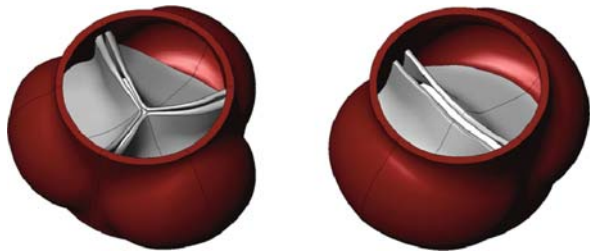
Fig. 16.11 Trileaflet ( left ) and bileaflet ( right ) geometries used in Weinberg and Mofrad [43]
