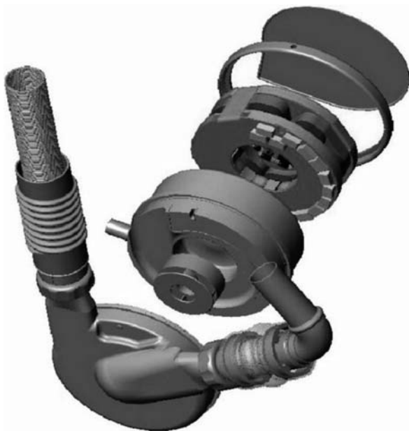
Fig. 18.5 Cross-section of the HeartMate III centrifugal pump. From Thoratec Corporation [16]
