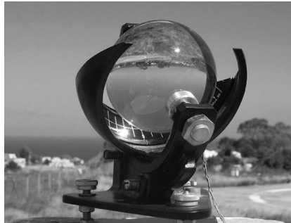
Figure 2.8. Typical Campbell–Stokes sunshine recorder (Image credit: http://commons.wikimedia.org/wiki/File:Heliografo.jpg )
