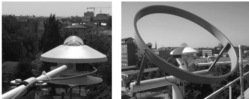
Figure 2.5. First-class pyranometers mounted on the Solar Platform of the West University of Timisoara, Romania: LPPYRA 05 measuring global and ground reflected solar irradiance (left) and LPPYRA 12 equipped with shadow band measuring the diffuse solar irradiance (right)
