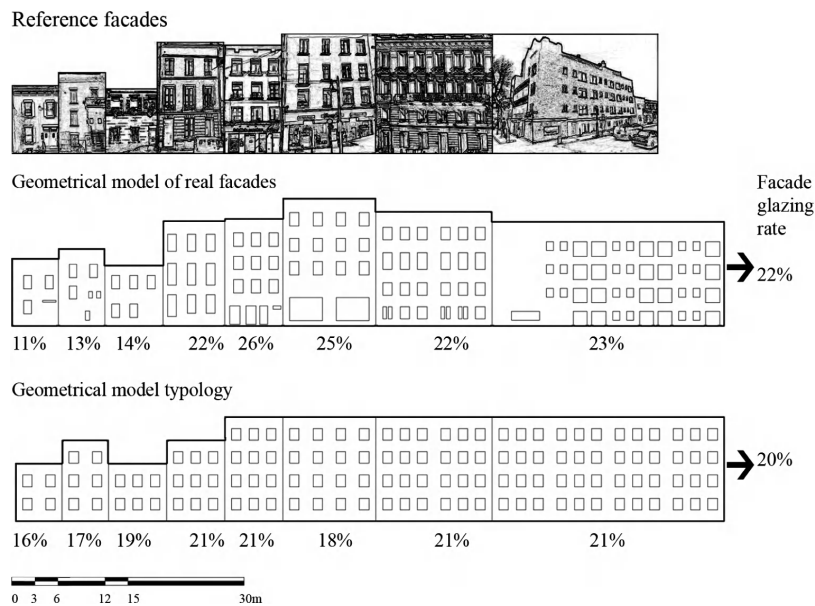
Figure 14.6. Definition of the facades of buildings types
