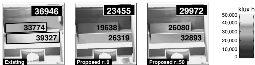
Figure 8.8. Total annual illumination incident at the skylights for the existing and proposed cases
