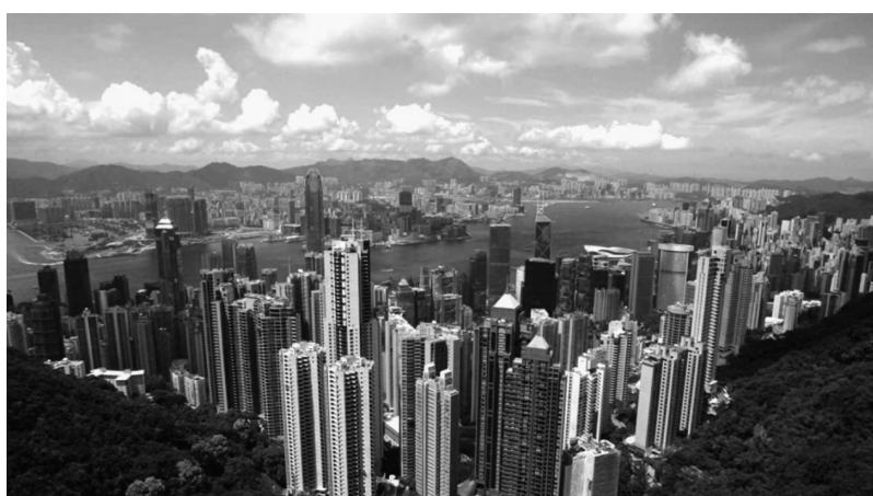
Figure 12.1. The cityscape of Hong Kong: closely packed buildings with high H/W ratio in the city can seriously limit the available daylight and solar access to indoor and outdoor spaces
