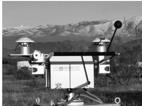
Figure 4.3. Two identical pyranometers, one for measuring GHI (on the left) and the other one shaded by a shadow-ball for measuring DHI (on the right). They are arranged in a sun-tracker to follow the apparent Sun path on the sky (Courtesy of V. Quaschnig, 2012 © www.volker-quaschnig.de )
