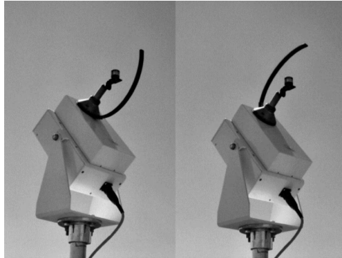
Figure 4.4. Pyranometer with a rotating shadow band. This pyranometer measures GHI while the shadow band is underneath, on the left, and DHI when the shadow band intercepts the beam component, on the right (Courtesy of V. Quaschnig, 2012 © www.volker-quaschnig.de)
