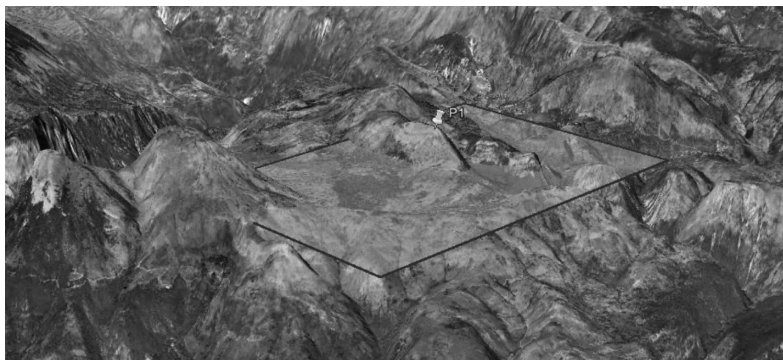
Figure 4.10. Sample of a cell in a solar radiation database. The horizontal area fenced is at the nominal altitude for this pixel by a given DEM. Nevertheless, the culminant point marked in the figure is well above the nominal altitude for this pixel. Other geographical points are well below
