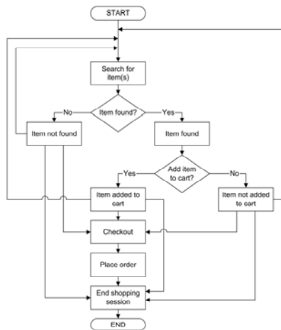
Fig. 6. The flowchart explaining the logic sequence of the e-Customer's behavior DSPN model
