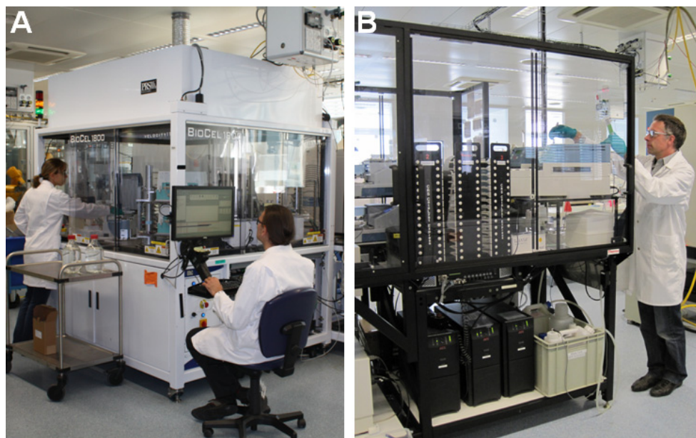
Fig. 2. Plate preparation platforms for automated HCS assays in 384 and 1536-well formats. A) Platform is used for compound addition, incubation and fixation. B) Platform is equipped with robot, dispensers, washers and incubators for automated antibody staining.
