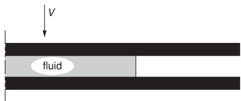
Figure 8.16. Schematic of axisymmetric squeeze flow. Reprinted from Debbaut, J. Non-Newtonian Fluid Mech. , 98 , 15 (2001). Copyright Elsevier.
