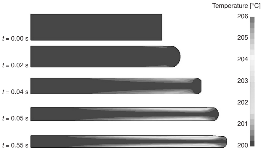
Figure 8.18. Shape and temperature evolution in time for adiabatic plates. Reprinted from Debbaut, J. Non-Newtonian Fluid Mech. , 98 , 15 (2001). Copyright Elsevier. For a color version of this figure, please go to the plate section.
