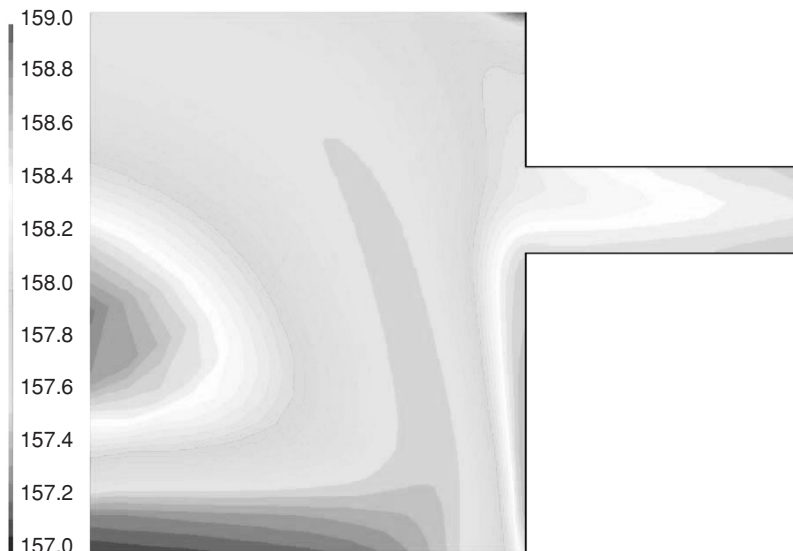
Figure 8.12. Computed temperature contours in the region near the die. For a color version of this figure, please go to the plate section.
