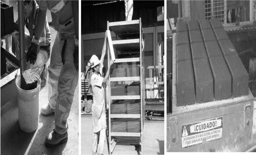
17.20 Concrete blocks for building construction and pavers, both made with slag-clinker hybrid cements.
