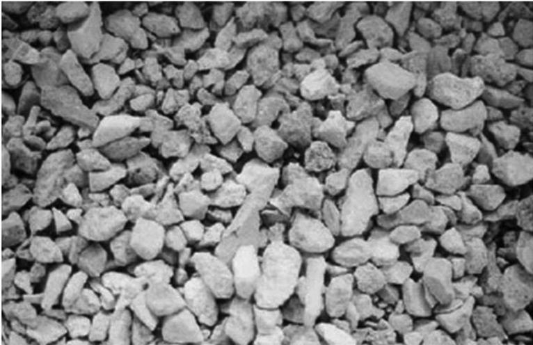
14.2 Recycled aggregates from masonry waste.
