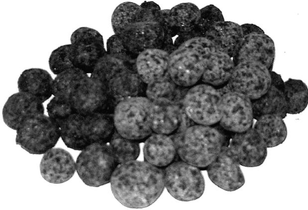
12.20 Artificial aggregates produced from MSWI bottom ash by sintering with other materials in a trefoil kiln. After Cresswell (2007).
