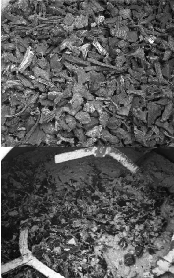
13.2 Rubber particles: top as they come after the shredding process; bottom, during the mixture of concrete (Aiello and Leuzzi, 2010).
