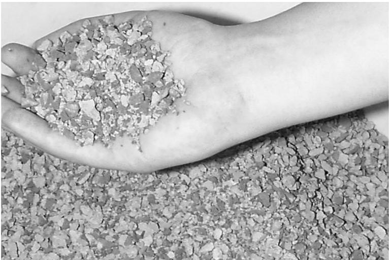
14.3 Recycled aggregates from concrete waste.
