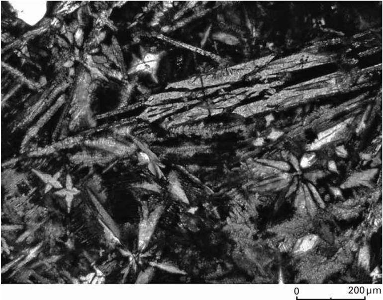
12.4 Hedenbergite (iron-rich clinopyroxene;  $\text{CaFeSi}_2\text{O}_6$ ) crystals in a MSWI bottom ash aggregate particle. Cross-polarized light. After Müller and Rübner (2006).
