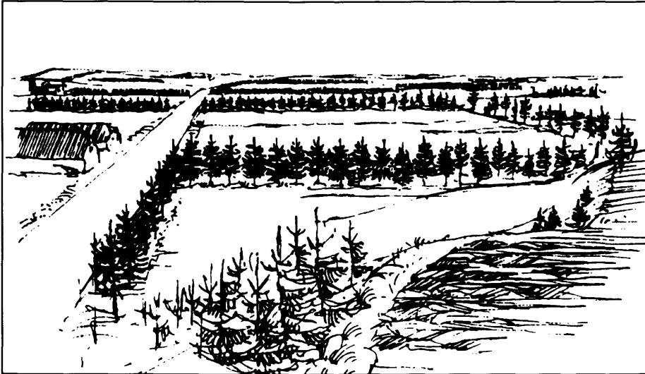
Fig. 3.8 Example of terrain with roughness length z_0 \approx 0.3 m. (After Petersen et al. (1980). Drawn by architect Søren Rasmussen. Reproduced by permission of Risø National Laboratory, Denmark).
