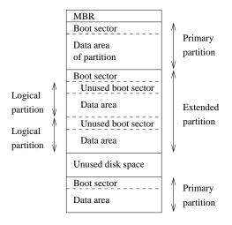
Figure 4.2: A sample hard disk partitioning.
