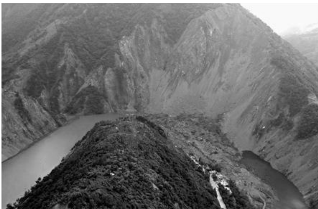
Fig. 3.11. Tangjiashan “quake lake” formed by landslide and mud blocking the Jianjiang River (31.643 Degrees, 104.429 Degrees) (Courtesy IEM)
