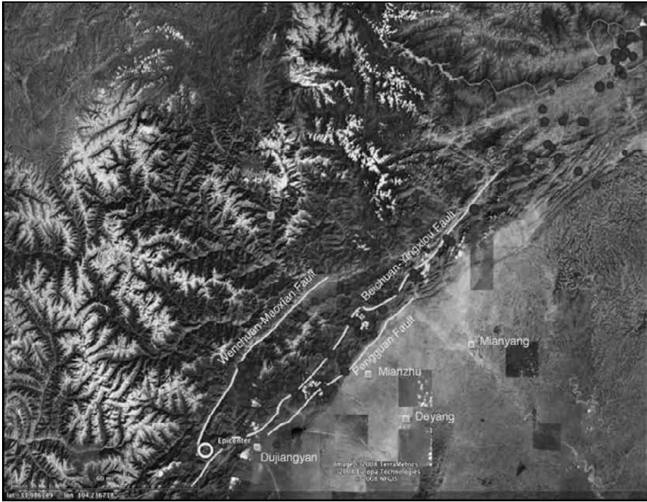
Fig. 2.6. Faults that ruptured on May 12, 2008; "O" marks the epicenter (Courtesy of IEM)
