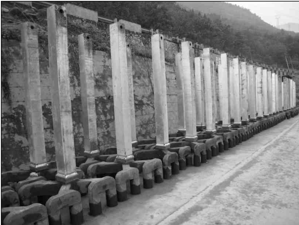
Fig. 4.24. Anodes for aluminum electrolysis
