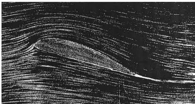
Figure 4.3 Photograph of the flow around a wing; the visualization was achieved by marked particles. From Prandtl and Tietjens (1931), Abbildung 47.
