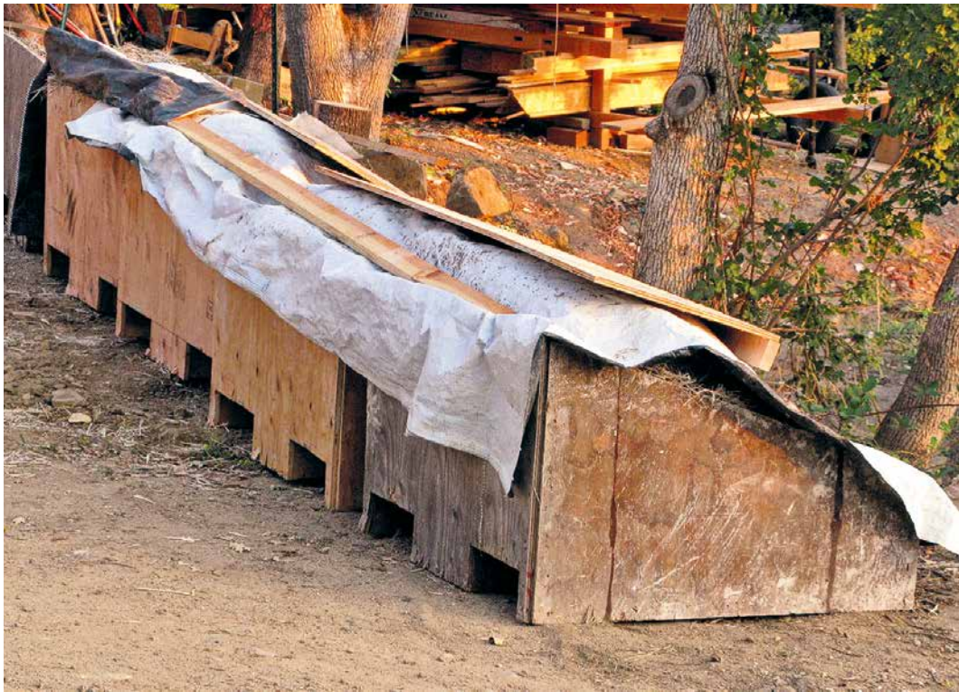
LSC curing in covered hoppers.
