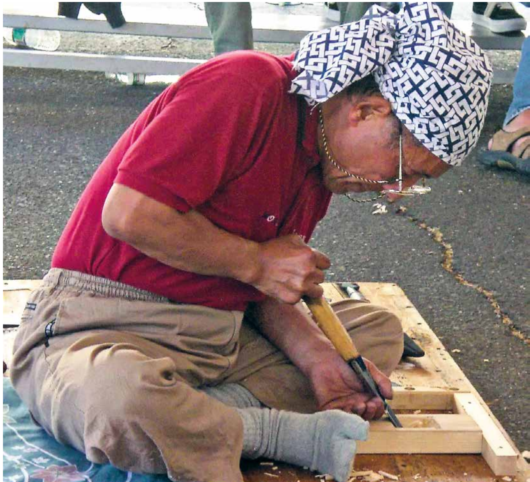
A master plane carpenter in traditional posture using all limbs to create a plane block.
