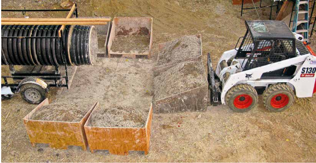
Hoppers in formation at discharge end of tumbler.
