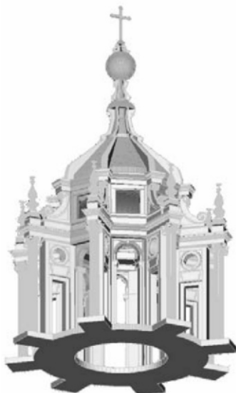
Axonometric projection of the lantern of S. Maria di Loreto by Giacomo Del Duca. Drawing by the author
