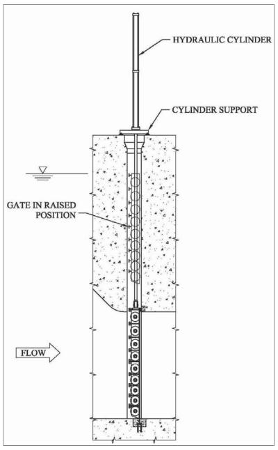
Figure 2-34. Wheel-mounted gate.
