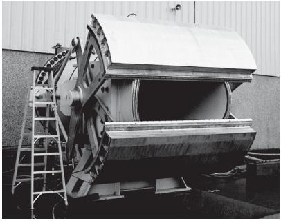
Figure 2-51. Clamshell gate before installation (Courtesy of USBR).
