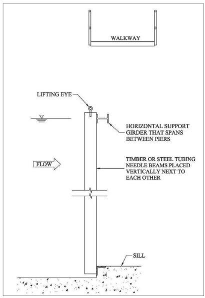
Figure 2-17. Needle beam system.
