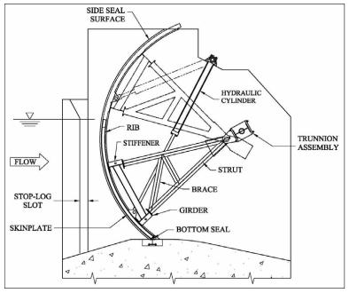
Figure 2-29. Hydraulically operated radial gate.
