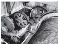
Figure 2-61. Exposed reduction gears.
