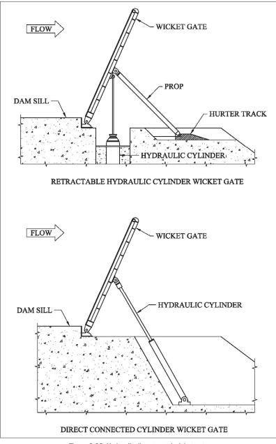
Figure 2-20. Hydraulically actuated wicket gate.
