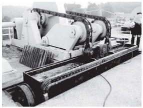
Figure 2-64. Roller Chain Hoist (Courtesy of TVA).
