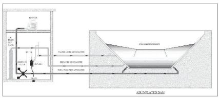
Figure 2-71. Mechanism for an air inflatable gate.
