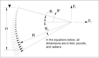
Figure 9-2. Curvilinear hydrostatic loads.
