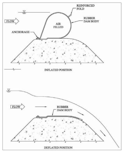
Figure 2-25. Rubber dam function.
