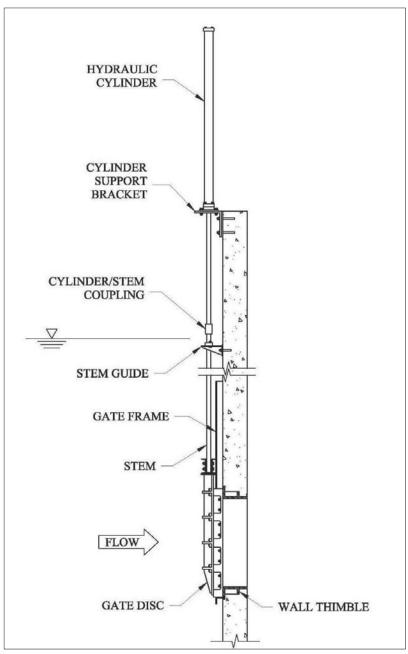
Figure 2-46. Sluice gate.
