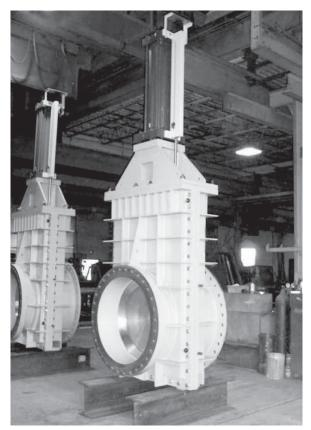
Figure 2-43. Jet-flow gates.
