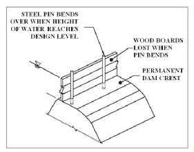
Figure 2-12. Pin type flashboards.
