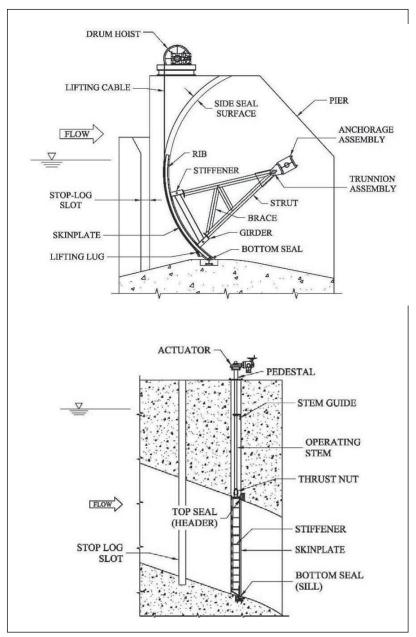
Figure 2-1. Basic gate components.
