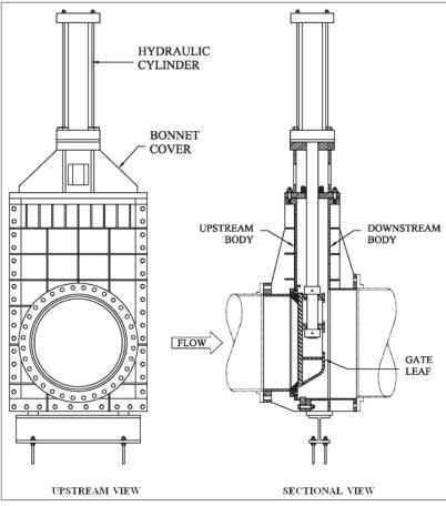
Figure 2-42. Jet-flow gate diagram view.
