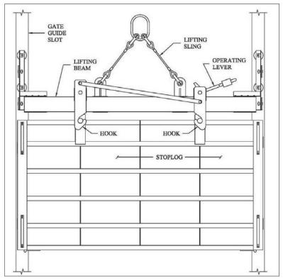
Figure 2-3. Stoplog with lifting beam.
