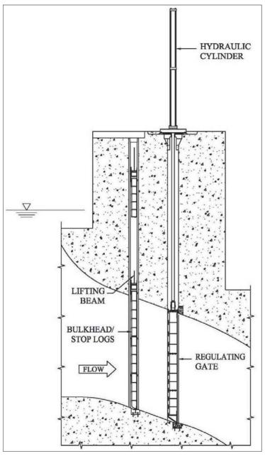
Figure 2-2. Bulkhead/stoplog.
