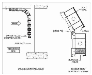
Figure 2-22. Articulated floating bulkhead.
