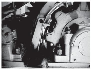
Figure 2-65. Chain Wheel (Courtesy of USACE).
