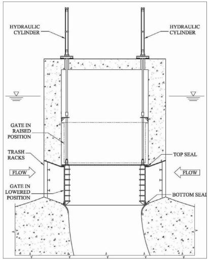
Figure 2-53. Cylinder gate.
