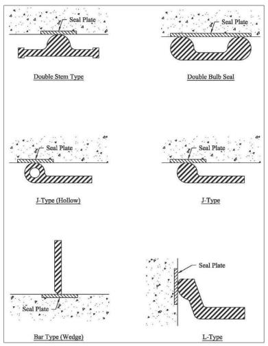
Figure 2-58. Common seal types.
