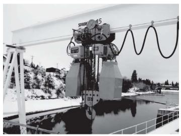
Figure 2-74. Motorized trolley on a monorail.
