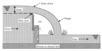
Figure 6.2 Side view of a weir.
