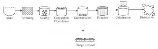
Figure 3.1 Unit processes: Water treatment.
