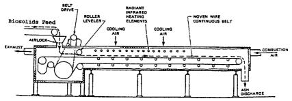
Figure 25.7 Cross section of an electric furnace. Source: USEPA, 1978, p. 15.
