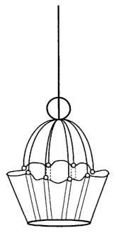
Figure 13.3 Debris catcher basket. Adapted from Parcher, M. Wastewater Collection Systems Maintenance. Lancaster, PA: Technomic Publishing Co., Inc., 1998, p. 248.
