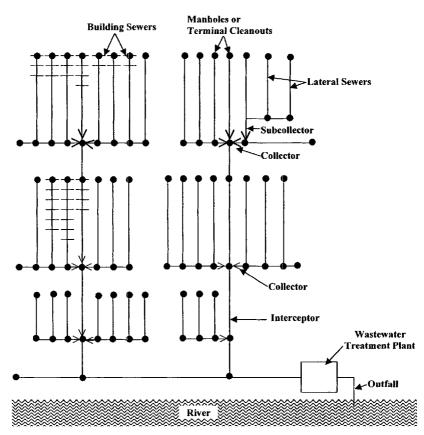
Figure 13.2 Collection system. Adapted from Qasim, S. R. Wastewater Treatment Plants, Planning, Design, and Operation, 2nd ed. Lancaster, PA: Technomic Publishing Co., Inc., 1999, p. 153.
