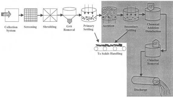
Figure 15.1 Unit processes for wastewater treatment: pretreatment.
