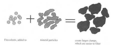
Figure 5.2 "Clumping" of particles.
