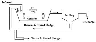
Figure 16.5 Activated sludge process (simplified).
