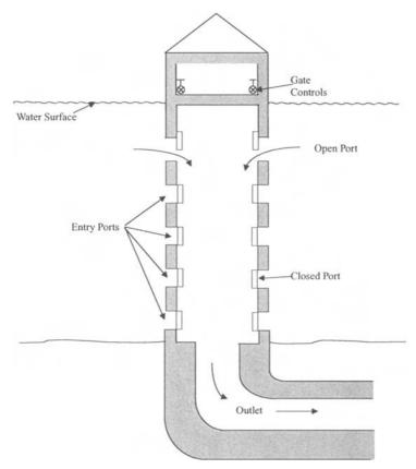
Figure 4.3 Tower water intake for a reservoir or lake water supply (larger than scale).
