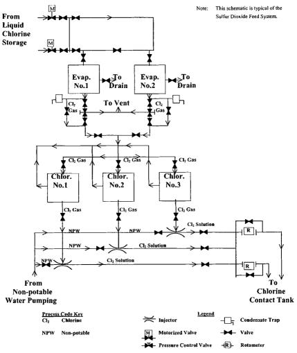
Figure 19.4 Disinfection chemical feeding process schematic diagram.
