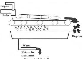
Figure 24.4 Belt filter press.
