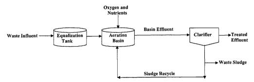
Figure 16.6 Activate sludge process.
