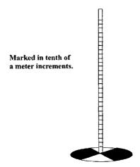
Figure 2.2 Secchi disk measures turbidity.
