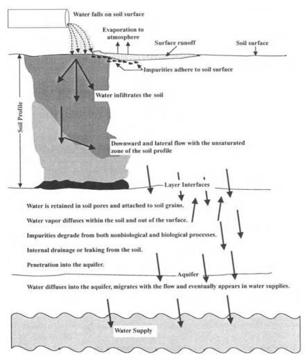
Figure 1.3 Movement of water through soil.
