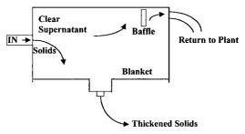
Figure 24.1 Gravity thickener.
