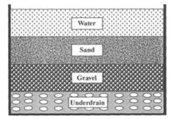
Figure 7.4 Rapid sand filter.
