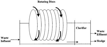
Figure 16.4 Rotating biological contactor.
