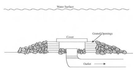
Figure 4.4 Submerged intake used for both lake and river sources.
