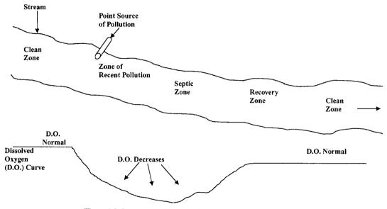
Figure 1.2 Stream zones (above) and dissolved oxygen curve (below).
