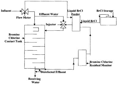
Figure 19.7 Bromine chloride feeder system.
