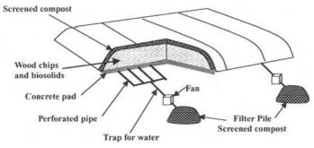
Figure 25.2 Aerated static pile.
