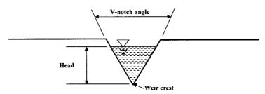
Figure 14.2b Triangular v-notch weir.
