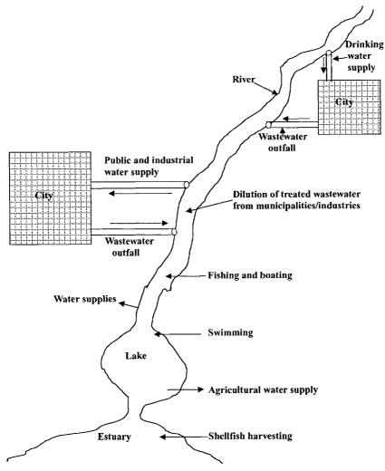
Figure 1.5 Indirect water reuse process.
