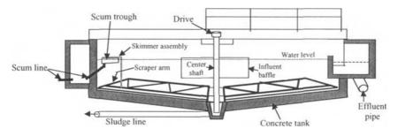
Figure 17.2 Sedimentation tank.
