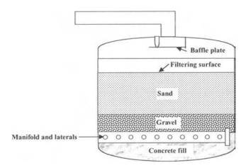
Figure 7.5 Pressure filter.
