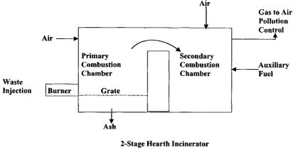
Figure 25.4 Hearth incinerator.
