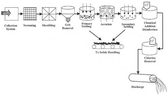
Figure 20.1 Unit processes for wastewater treatment: discharge.
