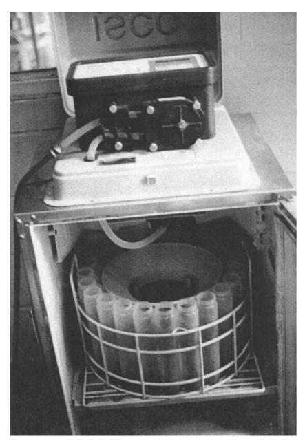
Photo 1.1 Automatic sampler (Lancaster, PA Advanced Wastewater Treatment Plant).
