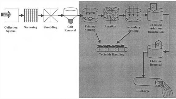
Figure 14.1 Unit processes for wastewater treatment: pretreatment.
