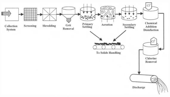
Figure 12.1 Unit processes for wastewater treatment.
