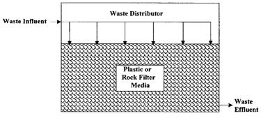
Figure 16.2 Trickling filter.
