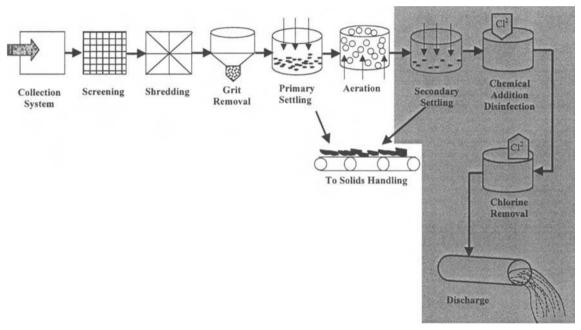
Figure 16.1 Unit processes for wastewater treatment: secondary or biological treatment.
