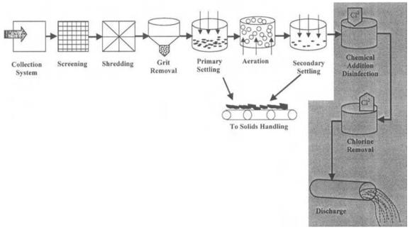
Figure 17.1 Unit processes for wastewater treatment: secondary sedimentation.
