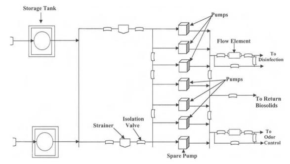
Figure 19.3 Process flow diagram sodium hypochlorite.
