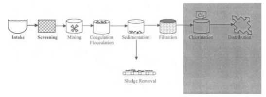
Figure 7.1 Basic water treatment unit processes: filtration added.
