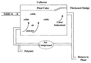
Figure 24.2 Flotation thickener.
