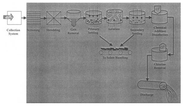
Figure 13.1 Unit processes for wastewater treatment: pretreatment.
