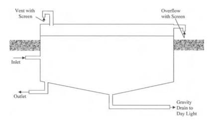
Figure 9.3d Ground-level service storage reservoir.
