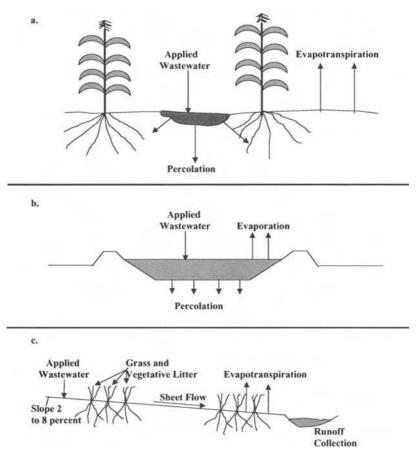
Figure 18.2 (a) Slow land treatment; (b) rapid filtration; (c) overland flow.
