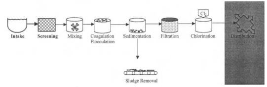
Figure 8.1 Basic water treatment unit processes: chlorination added.
