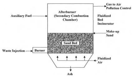
Figure 25.5 Fluidized bed incinerator.
