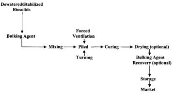
Figure 25.1 Flow diagram for composting biosolids.
