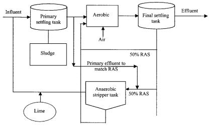
Figure 18.1 Sidestream process for biophosphorus removal.
