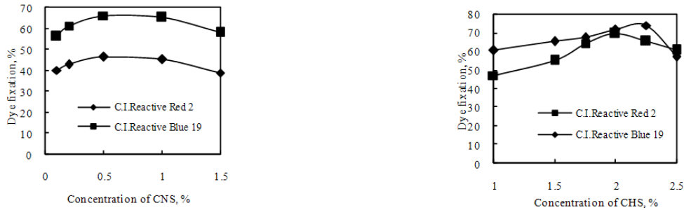
Fig.6. Effect of CNS concentration on dye fixation Fig. 7. Effect of CNS concentration on dye fixation
