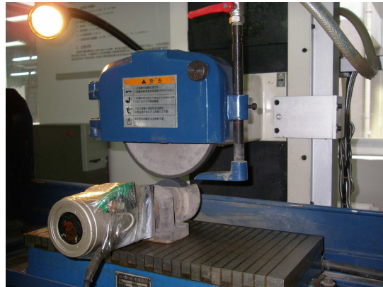
Fig.5. Photograph of truing and dressing the resin-bonded CBN wheel
