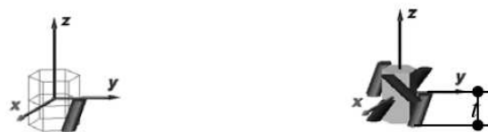
(a) A yarn segment (b) Combination of yarn segment corresponding to point group S_6 Fig.1 Deducing 3D braided geometrical structure unit-cell With space point group \bar{3}
