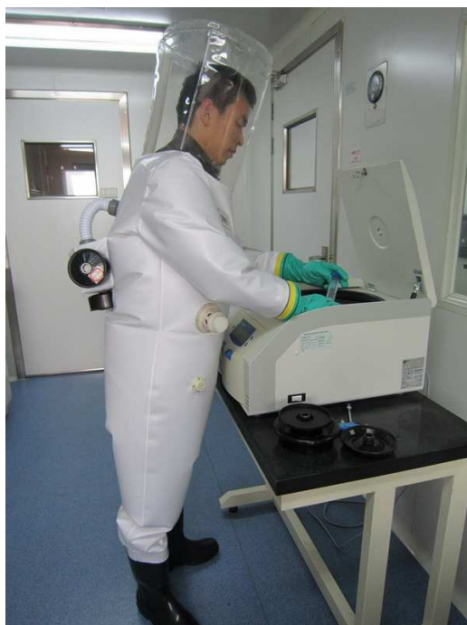
Fig 2 A kind of positive pressure bio-protection suit made of the polyurethane anti-bacterial composite fabric
