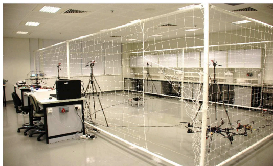
Fig. 2 Safety net outlining the Qball-X4 workspace.
