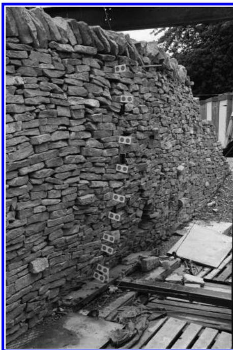
*Figure 3.9* A well-developed bulge in a test wall. This bulge went on to collapse when the load plate on the backfill was pushed further.
