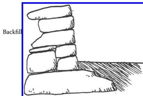
Figure 5.17 Foundation stones larger than the thickness of the wall, providing a footing (the origin of the term is obvious in this illustration).
