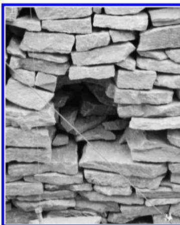
Figure 6.8 Part of a test wall at the University of Bath. A section of facing stone has fallen away completely.
