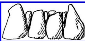
Figure 5.27 Wedges hold the back ends of the stones in place – view from above.
