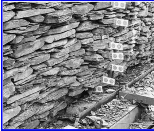
*Figure 6.12* A test wall at the University of Bath constructed from shale. This wall failed in sliding. The targets enable the distance the wall had slid on its base to be seen clearly; this photograph was taken just before the wall failed.
