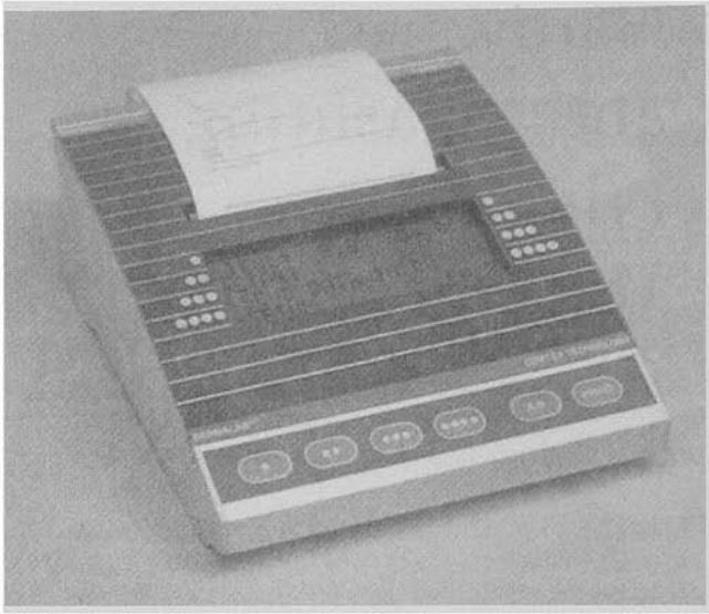
FIGURE 10.1 The DermaLab skin elasticity measurer. The complete DermaLab system also includes systems and probes for measurement of transepidermal water loss and epidermal hydration. (Courtesy of Manufacturer Cortex Technology, Hadsund, Denmark.)
