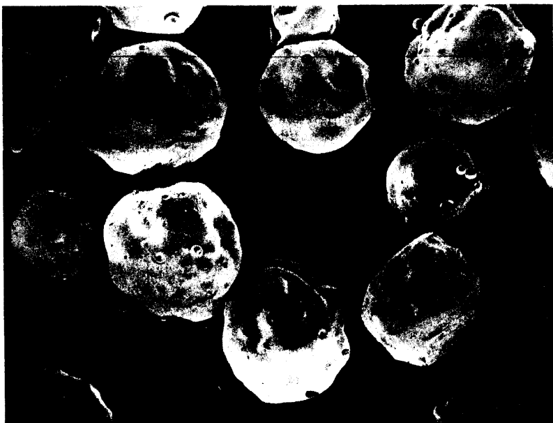
FIGURE 12 Scanning electron micrograph of contraceptive vaccine microspheres based on lactide/glycolide polymer.
