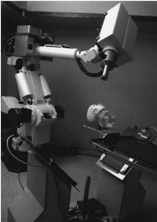
FIGURE 1 A picture of the Cyberknife showing the linear accelerator, the robotic arm, the treatment couch, and the amorphous silicon x-ray cameras (mounted on the floor). Reprinted with permission from Adler JR, Murphy MJ, Chang SD, Hancock SL. Image-guided robotic radiosurgery. Neurosurgery 44:1299–1307, 1999.
