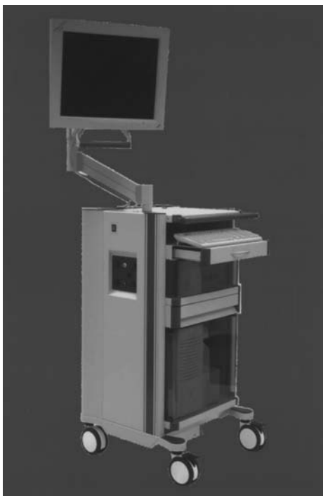
FIGURE 1 Voyager system composed of dual CCD camera, equipment rack with extendable flat panel liquid crystal display (LCD), and outboard flat panel LCD display.
