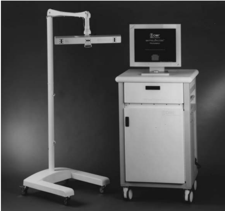
FIGURE 1 The Mayfield ACCISS system. Custom computer cart and infrared camera for optical tracking.
