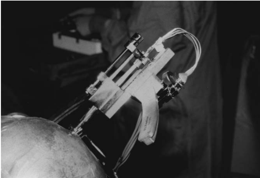
FIGURE 2 Microdrive mounted in the localizing unit of the Zamorano Dujovny (Z-D) frame. The neurosurgeon can change the position of the microelectrode intraoperatively.
