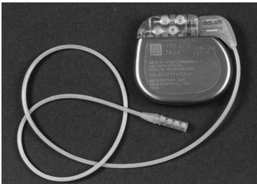
FIGURE 2 Fully implantable and programmable pulse generator, Itriel-II with its extension cord. (Courtesy of Medtronic, Inc.)
