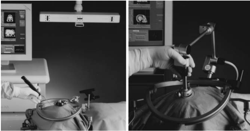
FIGURE 2 The Mayfield ACCISS dual digitizing system. Left , wireless active optical tracking systems with infrared camera. Right , mechanical arm system with the tip of the mechanical arm in the AccuPoint sphere for stereotactic targeting.
