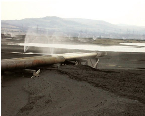
Fig. 8.35 Spray irrigation of tailings surface to prevent wind erosion
