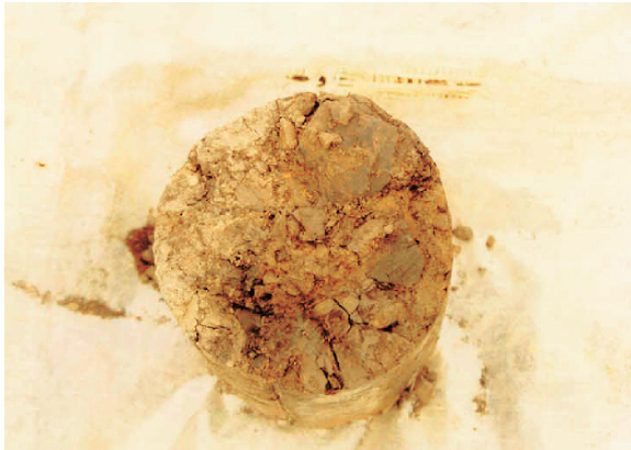
Fig. 8.12 Heterogeneity of spoil heap, (according to Větrovský). (a) boring core from the depth 34 m. (b) core from smaller depth
