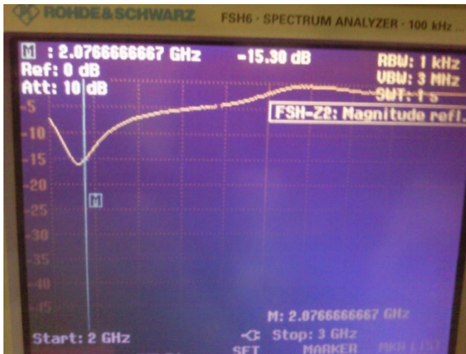
Fig. 6. Measurement of return loss S11=-15.30 dB
