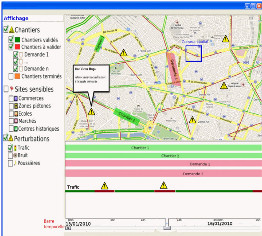
Fig. 3. This figure shows how the system displays traffic information both in spatial and temporal windows. Alerts are represented by graphical indicators. When these indicators are pointed, the corresponding warnings are displayed.
